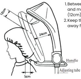
1.Between the top point of client's head and machine's rotation center, a 5" (12cm) distance should be reserved
