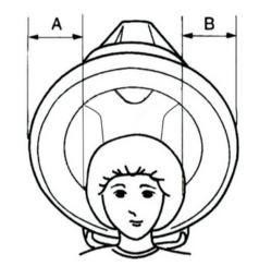
Keep distance A and B the same (as shown above), in order to keep client in the middle of the machine.
