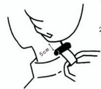
1. Set height by adjusting the supporting tube to place the rubber piece behind client's neck.
