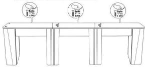
Install Bolts from the inner side of the marble table onto the marble top \_Each side fit 1 bolt (1"1/4 x3)
