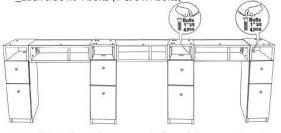
Install Bolts from the inner side flap of the two side cabinet tables \_Each side fit 4 bolts (1"3/8 x4 bolts)
