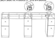
Install Bolts from the inner side flap of the two side cabinet tables \_Each side fit 4 bolts (1"3/8 x4 bolts)
