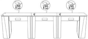
Install Bolts from the inner side of the marble table onto the marble top \_Each side fit 1 bolt (1"1/4 x3)
