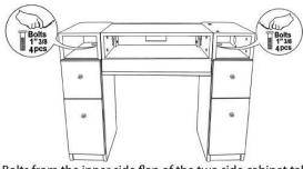
Install Bolts from the inner side flap of the two side cabinet tables \_Each side fit 4 bolts (1"3/8 x4 bolts)
