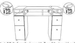
Install Bolts from the inner side flap of the two side cabinet tables \_Each side fit 4 bolts (1"3/8 x4 bolts) \_\_\_
