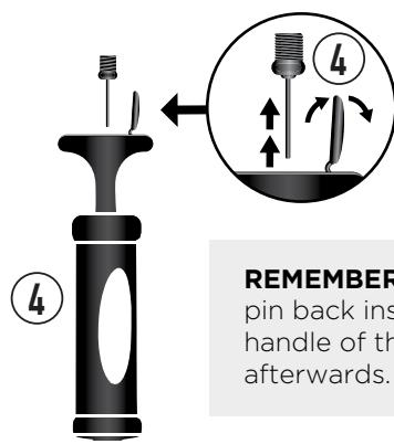
**REMEMBER:** place the pin back inside the handle of the pump afterwards.
