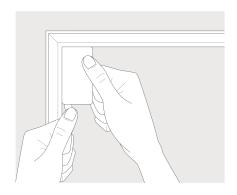
TIP: If you find that the brackets are difficult to place behind the window seal, you can use a some washing up liquid as lubricant on the flat part of the bracket. Once all the brackets are fitted, clean any excess from the window surface.
