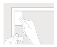
TIP: You can use a credit/debit card as template to find the correct position for the brackets. Place the card length ways along the side of the window in each corner, and line up the bracket with the end of the card as shown.
