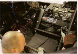
Now with all the speakers installed it's time to add some bass and the amp. The storage area underneath the driver's seat is the perfect mounting position. Simply undo the 4 screws holding on your cross piece for your seat base and slide in the 10" sub box. The amp will mount on top of the box and you'll have about 2" of clearance between the top of the amp and the seat seat base. Like a glove.
