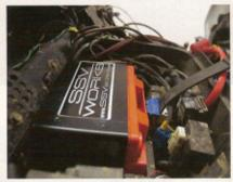
You'll want some more juice to power your system, especially if you're going to run your stereo without the machine running. This dry cell battery fits right into your stock location.
