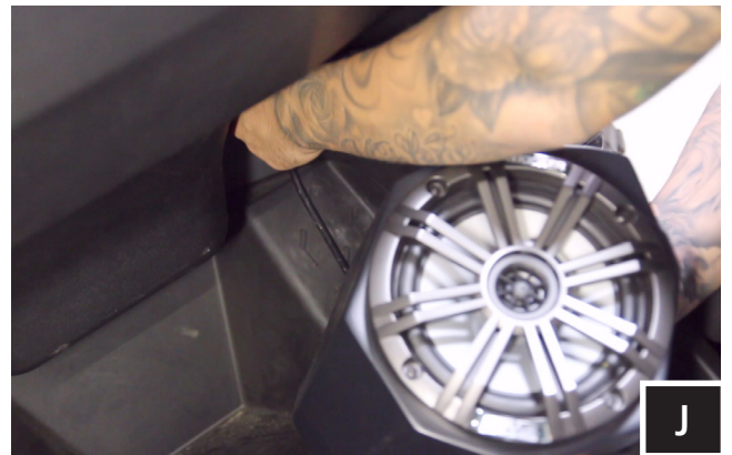
J. Route speaker connector through the 1/2" hole that was drilled out.
