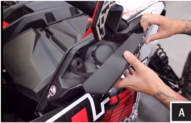
A. Front covers will need to be removed, start by removing passenger side gas cover.
