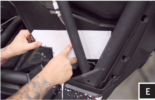
E. Cut out the template (Driver/Passenger) along the cut line. Position the template on inner plastic, making sure to square up the template along the factory panel as shown in image E.
