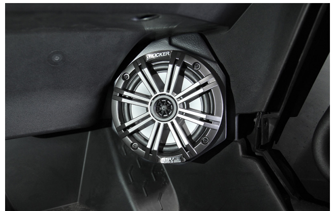
Installation is complete. Repeat for driver side pod.
