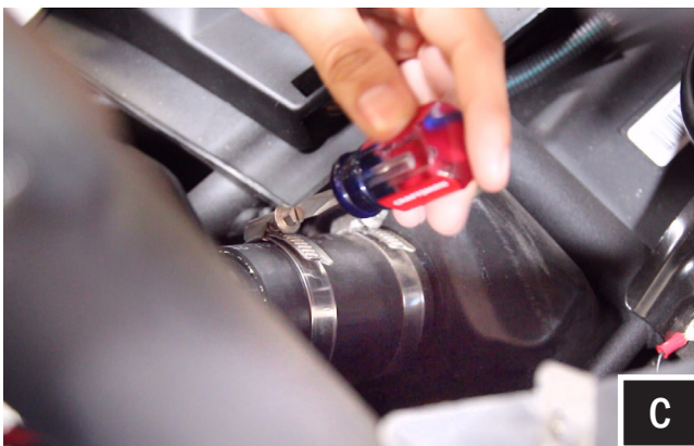
C. Using a flat head screw driver to loosen the hose clamp on the gas tube. Note: You will have to remove three (3) additional T30 screws holding the top OE speaker pod cover for access to gas clamp.
