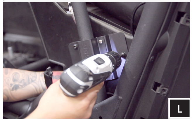
L. Once all screws have been inserted into pod, tighten all three (3) screws.
