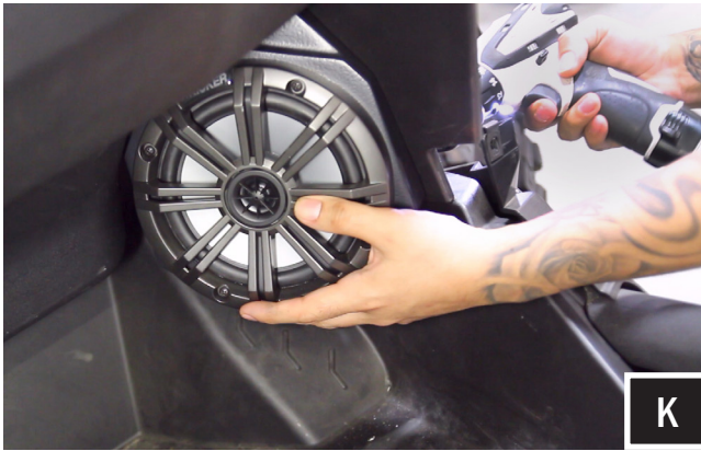
K. Place the kick pod in position for mounting. Use the provided M6 screws and washers to hand tighten the pod to the kick panel.
