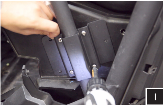
I. Place the smaller bracket on top of the bar and line up the holes with the large bracket. Using the M5 screws, tighten both brackets to one another (make sure the drilled out holes line up to brackets)
