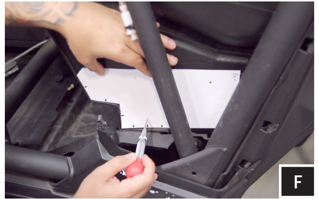
F. Using a scribing tool, mark the center of the three (3) drill points illustrated on the template as shown in image F.
