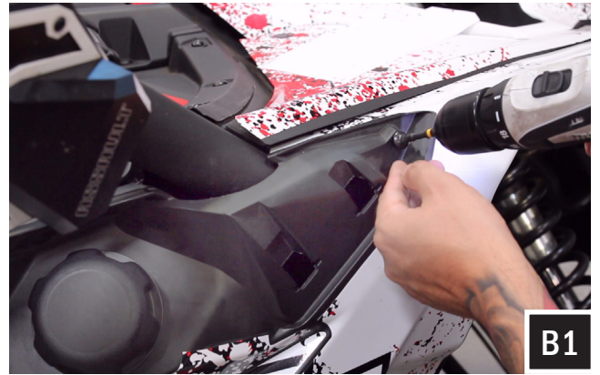
B. Remove the eleven (11) T30 Torx bolts that secure the fender. Note: There is three (3) T30 screws on passenger side and two (2) on driver side that will have a 10mm bolt. Remove the metal clip that is securing the top panel to the fender.
