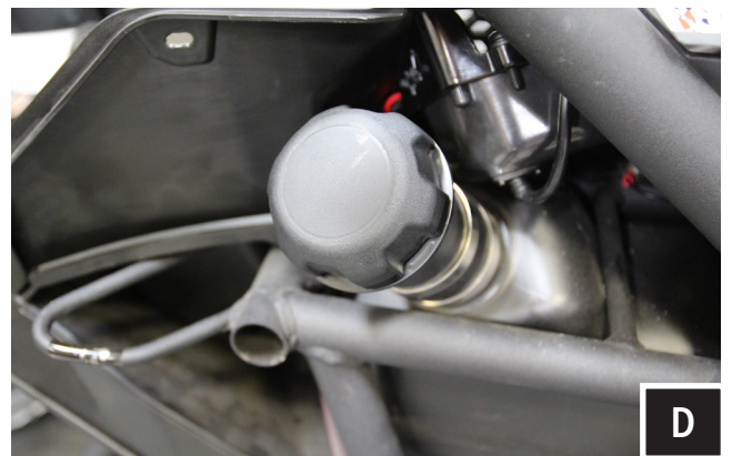
D. Remove gas tube from fender and place back on gas tank until install is complete
