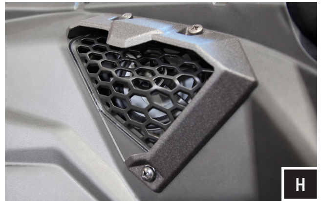
H. Route the speaker wire away from any moving parts and any sharp metal, then connect to the amplifier. Connecting the X3-D4 using the pre-installed, two-pin connector will require an optional SSV Works plug-&-play harness (WP-H1149 - sold separately). If you are not using the WP-H1149 harness, simply cut off the two-pin connector and follow the wiring instruction below.
