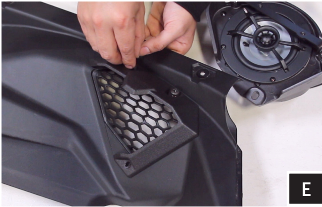
E. Place the acoustic lens on top of the factory grille, line up the holes and insert the 2 top M6x1.0 (shorter) screws and washers.
