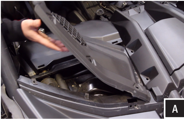
A. Remove the top dash panels on the driver (7 screws with 2 clips) and passenger side (5 screws with 2 clips).
