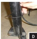
D. Using the zip ties provided, route the Power/Ground loom to the battery location away from any moving parts or sharp metal. NOTE: The 4 pin long cable is an audio output for adding an additional amplifier and speakers.
