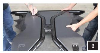
B. While holding the enclosure securely to the underside of the cage, loosely install the 5 brackets using the screws provided, attaching the front brackets first will help support the enclosure while attaching the other brackets
