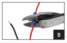
B. Crimp the supplied fuse holder onto the end of the RED wire and attach to the battery "+" terminal.
