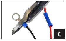
C. Crimp the supplied ring terminal to the BLACK wire and attach to the battery "-" terminal.
