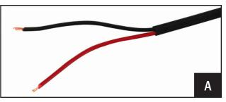
A. Cut the power/ground cable to length; be sure to leave enough wire at the battery location to wire to the battery, strip back approximately 4 inches of the black tubing to expose the red/black wires inside. Strip back 1/4"-1/2" of wire to make your connections.
