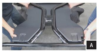
A. With one person on either side of the vehicle place the WP3-WC2O4A into location from the underside of the cage, place the back into position first, and then swing the front up into place.
