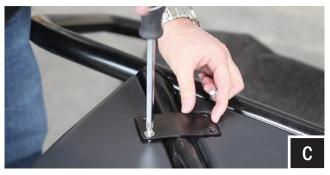
C. Once the enclosure is in position, tighten the brackets using the #3 screwdriver. NOTE: After all brackets are tightened, it may be necessary to go back and re-adjust the brackets to ensure the enclosure is properly secured.
