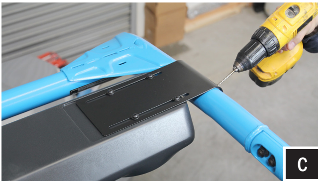
C. With the WP3-U04SA in the proper mounting location, pre drill the bracket mounting holes using the 1/8" drill bit, use the holes in the bracket as a guide.
