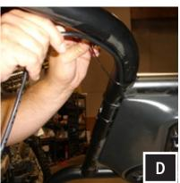
D. Using the zip ties provided, route the Power/ Ground loom to the battery location away from any moving parts or sharp metal. NOTE: The 4 pin short cable is for additional speakers (WP3-RZOA+2) and the 4 pin long cable is for adding an SSV Works Powered Subwoofer (Part# WP-RZS10)
