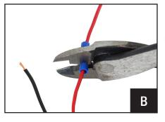
B. Crimp the supplied fuse holder onto the end of the RED wire and attach to the battery "+" terminal.
