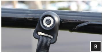
B. The enclosure brackets will utilize one safety net bolt on each side. Remove both with a 10mm socket.
