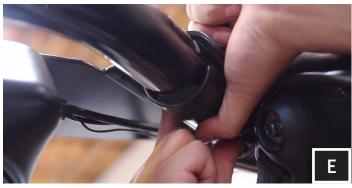
E. Install both bottom J Brackets using (4) Phillips screws (8) Washers and (4) lock nuts. Be sure rubber insterts are pre-installed.
