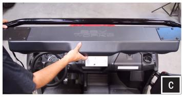
C. Place the WP3-PN3O4A onto the cage with the (2) J style brackets resting on the front of the cage.
