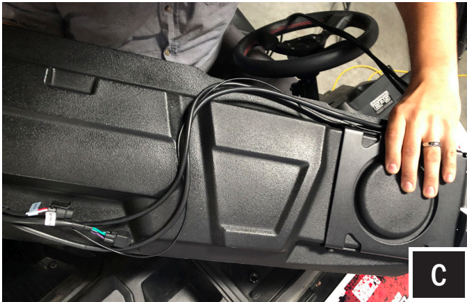
C. Guide the harness over the top of the enclosure and out the driver side.
