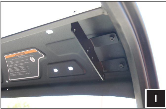
I. With the stereo removed, reinstall the roof.
