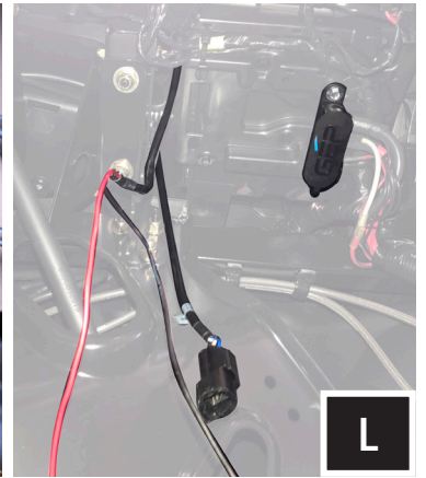
L. Route the power/ground and ext. amp trigger output into the dash cavity. Once in the dash cavity, pull the power/ground and ext. amp trigger output across the dash cavity along the factory harnesses to the bus bar.
