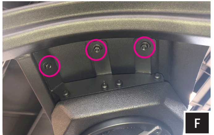
F. From the inside the cab fasten a M6 washer and nut onto each M6 screw.
