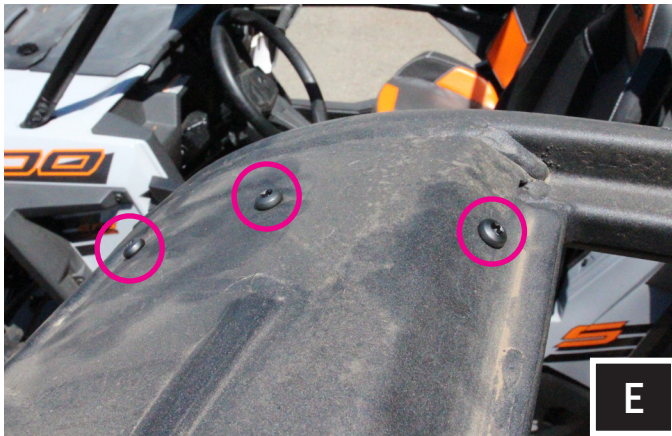
E. From the top of ROP visor, place (3) M6 T30 torx screws per side through the visor and stereo mounting brackets.
