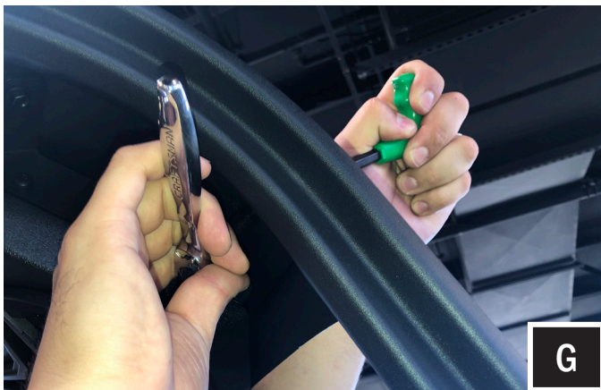
G. Using a T30 torx driver and 10mm socket, tighten all (6) M6 screws to secure the stereo to the ROP visor. If you are not installing a roof, skip to Step K.
