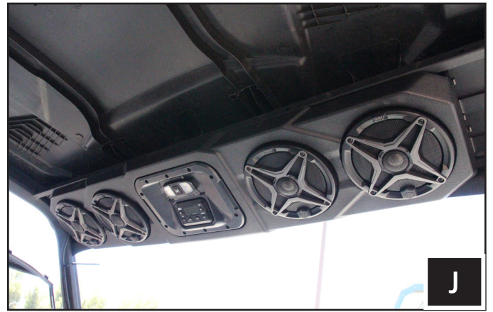
J. Guide the harness out the driver side. Lift the enclosure back into place and fasten the stereo back to the mounting brackets with the (8) M6 t30 Torx screws.
