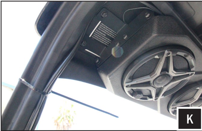
K. Guide the harness out the driver side. Fasten the stereo back to the mounting brackets with the (8) M6 T30 Torx screws.
