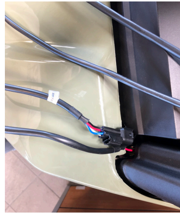
L. Route the power/ground and ext. amp trigger output into the dash cavity. Once in the dash cavity, pull the power/ground and ext. amp trigger output across the dash cavity along the factory harnesses to the bus bar.
