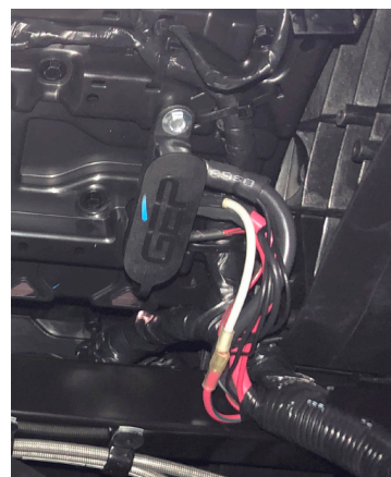
N. Pull guard away from bus bar, remove the 10mm nut on the 2nd position terminal for 12v constant power or the 1st position for accessory power and attach the red POWER wire. Refasten on the nut. Remove the 10mm nut on the 3rd position terminal and attach the black GROUND wire. Refasten on the nut.
