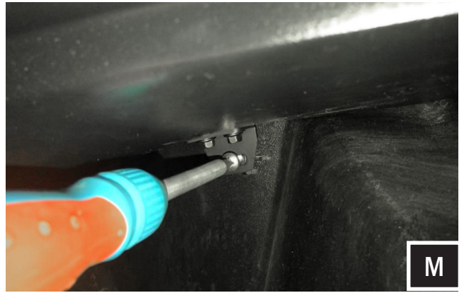
M. Fasten the provided #14 screw to secure the enclosure lower mounting bracket.
