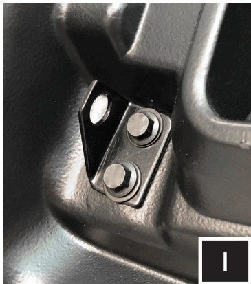
I. Install left and right door hinge brackets using (2) 8mm screws and washers for each side.
