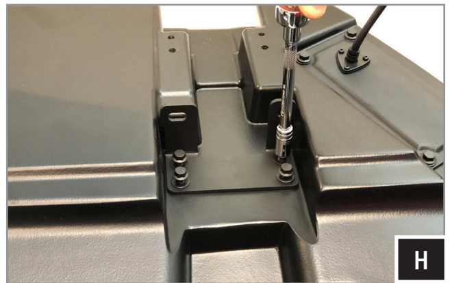
H. Using (4) 8mm screws and washers, attach Bracket "B" to the enclosure.
