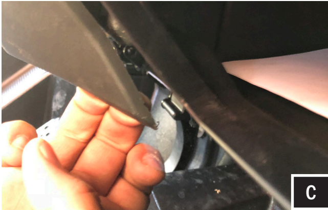
C. Unclip the dash surrounding the glovebox. Once unclipped, gently pull the dash forward and remove the upper dash pocket.
