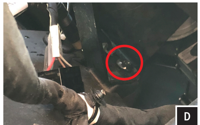
D. Extract the (1) T40 torx that secures the lower dash pocket
