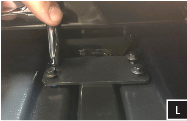
L. Place Bracket "A" into place towards the firewall, and fasten it into place with the (4) 8mm socket head screws and washers provided with the kit.
