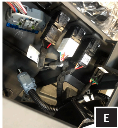
E. Disconnect the USB and unclip the LED from the lower dash pocket. Remove the lower dash pocket. Label / take photos of the harnesses connected to the dash. Once recorded, disconnect harnesses, and remove dash.
