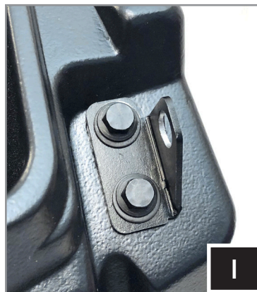
I. Install left and right door hinge brackets using (2) 8mm screws and washers for each side.
