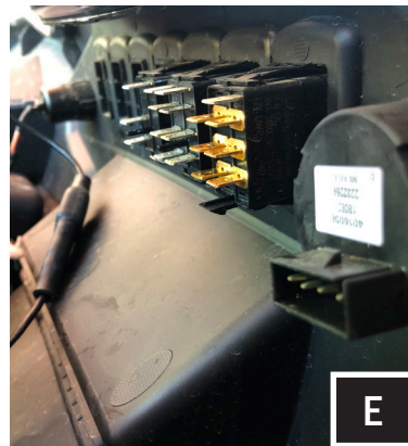
E. Disconnect the USB and unclip the LED from the lower dash pocket. Remove the lower dash pocket. Label / take photos of the harnesses connected to the dash. Once recorded, disconnect harnesses, and remove dash.
