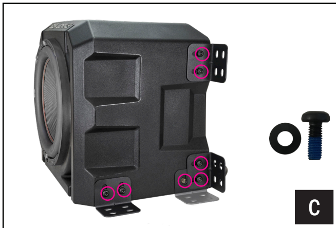
C. Depending on installation location, attach all four mounting brackets on the bottom installation position or the back installation position. Use M6x16mm Button Head Torx Screws and M6 Washers to secure the brackets.
