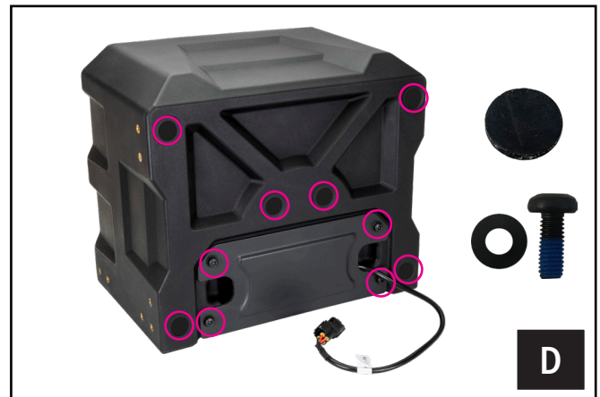
D. Attach Amp Cover to Enclosure using four M6x16mm Torx Screws and M6 Washers. Route Sub Wiring through hole cut. Attach all six Vibration Absorption Pads to the back or bottom, depending on which position you orient the enclosure into your vehicle.
