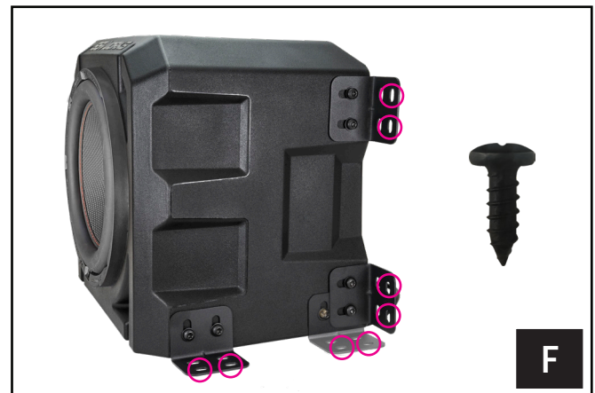
F. Depending on installation location, attach all four mounting brackets on the bottom installation position or the back installation position into the vehicle. Use 10 x .75" Screws to secure the sub enclosure into the vehicle.
