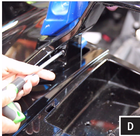
D. Remove driver and passenger side panels that cover the roll bars. Use T40 torx screwdriver to remove the front and back screws and a T25 torx to remove the screws underneath top of panel.
