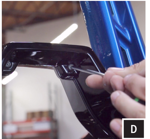
D. Remove driver and passenger side panels that cover the roll bars. Use T40 torx screwdriver to remove the front and back screws and a T25 torx to remove the screws underneath top of panel.
