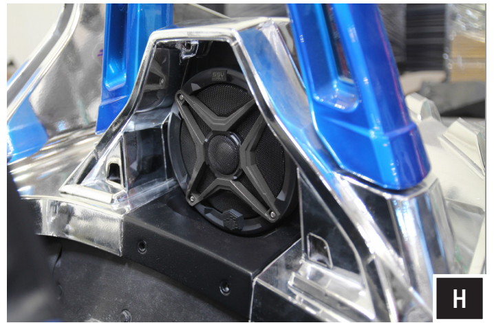
H. Re-install gas cap nut (driver side only). Re-install gas cap (driver side only). Re-install screws in the front of the speaker pod (2 places). Re-install headrest frame.
