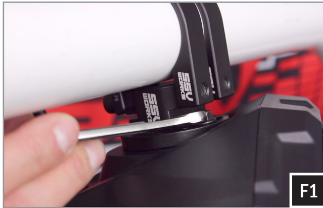
F1. Position the speaker to your liking and tighten the 8mm hex screws.
