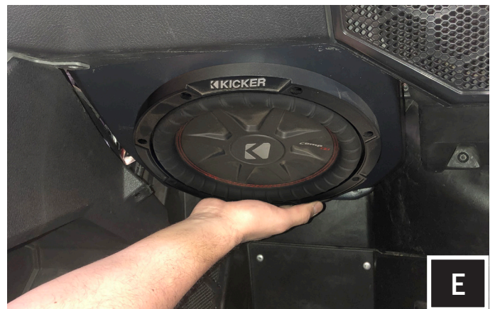
E. Apply force to the bottom of the enclosure to swing it into place. Once it is in place the lower mounting points will be in-line with the (2) M6 clip nuts.
