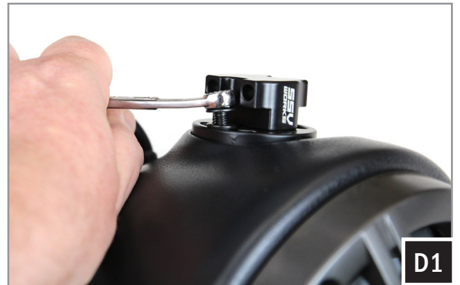
D1. Loosely install the clamp base to the US-C65A with (2) M6x1.0x20mm screws and washers using a 8mm open-ended wrench. Position the clamp base to your desired position and tighten the (2) M6x1.0x20mm screws.
