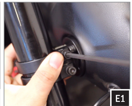
E1. Wrap a plastic bag around the roll cage to prevent scratching. Press the clamps onto the roll cage over the plastic bag. Place the (2) M6x1.0x45mm screws and washers through the clamp and clamp base. Secure the clamps to the roll cage with a 5mm allen key.
