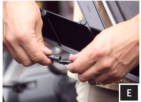
E. Route the B-H2195 Driver and passenger cables to their assigned speaker pods. Connect the B-H2195 to the door pod cable.
