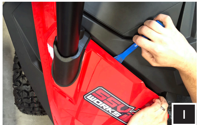
I. Use a panel to aid in lifting the fenders to release the top dash panel.
