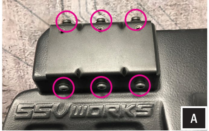
A. Secure the base bracket to the enclosure with (6) M6x1.0x12mm T30 screws and washers.
