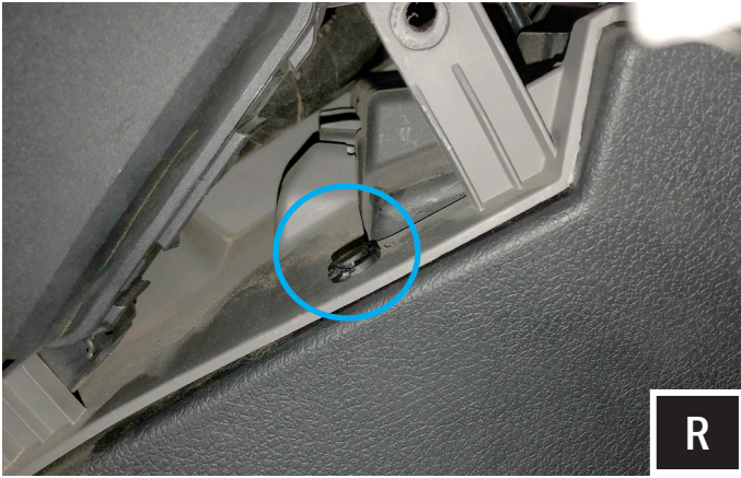
R. Rotate the fuse block counterclockwise and remove the now exposed push pin.
