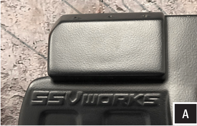
A. Secure the base bracket to the enclosure with (6) M6x1.0x12mm T30 screws and washers.
