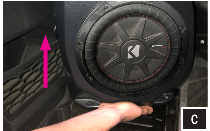
C. From the Passenger footwell, lift the RZ5-UD10 into the dash cavity.
