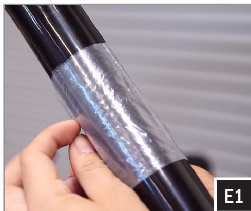
E1. Wrap a plastic bag around the roll cage to prevent scratching. Press the clamps onto the roll cage over the plastic bag. Place the (2) M6x1.0x45mm screws and washers through the clamp and clamp base. Secure the clamps to the roll cage with a 5mm allen key.
