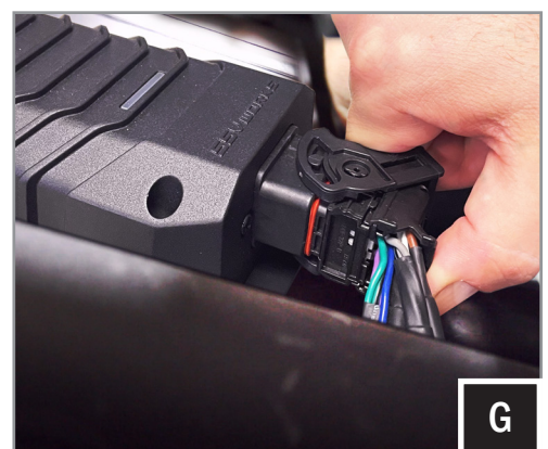
G. Connect the INPUT and OUTPUT Harness into the 800.5 amp. Connect ground wire to billet connector that the factory amp was plugged into when it was removed.
