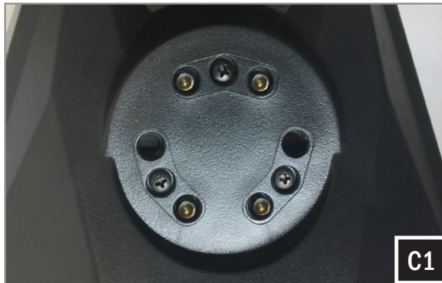
C1. Find your desired orientation for the US-C65A on your roll cage and fasten the set screws with a 3mm allen key in the opposite holes of where the clamp will install two.
