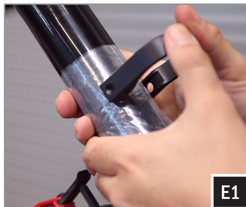
E1. Wrap a plastic bag around the roll cage to prevent scratching. Press the clamps onto the roll cage over the plastic bag. Place the (2) M6x1.0x45mm screws and washers through the clamp and clamp base. Secure the clamps to the roll cage with a 5mm allen key.
