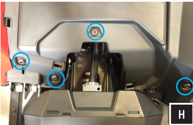
H. Remove the (4) T40 Torx screws that surround the gauge cluster. For ease of access to each screw we recommend adjusting the position of the steering column accordingly.
