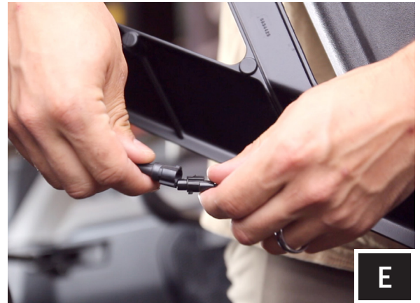
E. Route the B-H2195 Driver and passenger cables to their assigned speaker pods. Connect the B-H2195 to the door pod cable.
