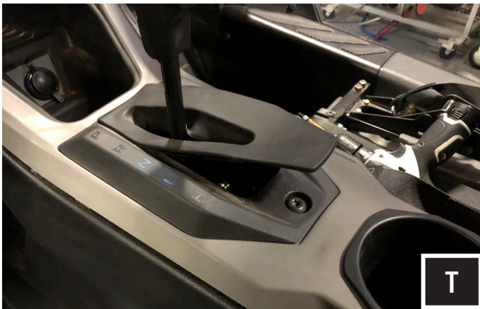
T. Lift the shift boot to expose the (1) T40 screw for removal
