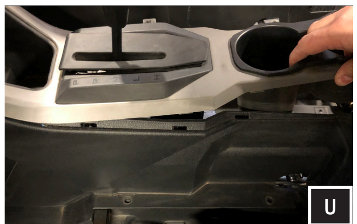
U. Gently lift center console to release/separate driver and passenger console side panels
