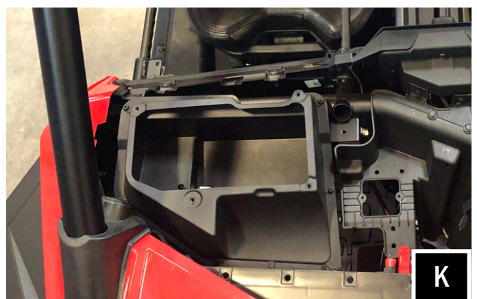
K. Lift and remove the glove compartment from the dash cavity.
