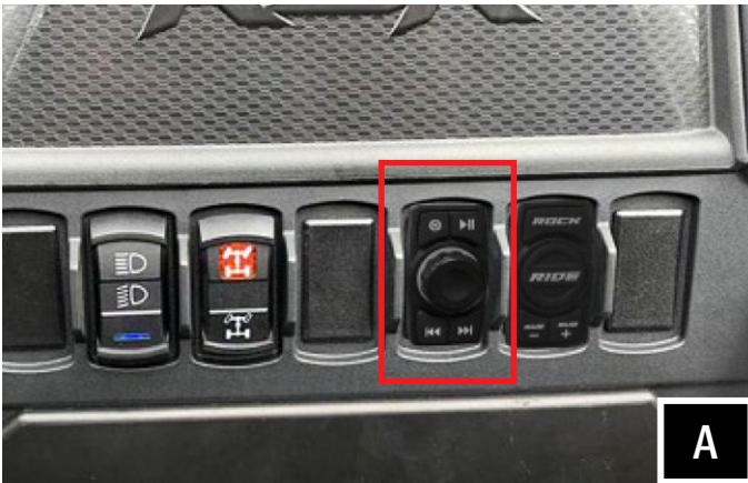
A. Pop out Rocker Switch cover and fish through the MRB2R Rocker Controller cable. Push in the MRB2R Rocker controller to secure in place.
