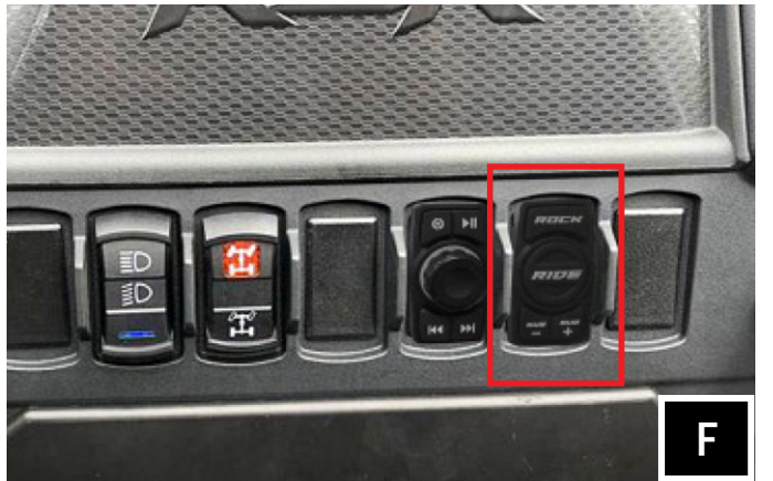
F. Pop out rocker switch cover and push in the Rock and Ride controller in your preferred location.
