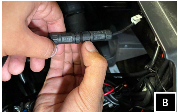
B. Carefully line up the plugs on the MRB2R Rocker Controller and Media Receiver, push them together and tighten hand screw nut.
