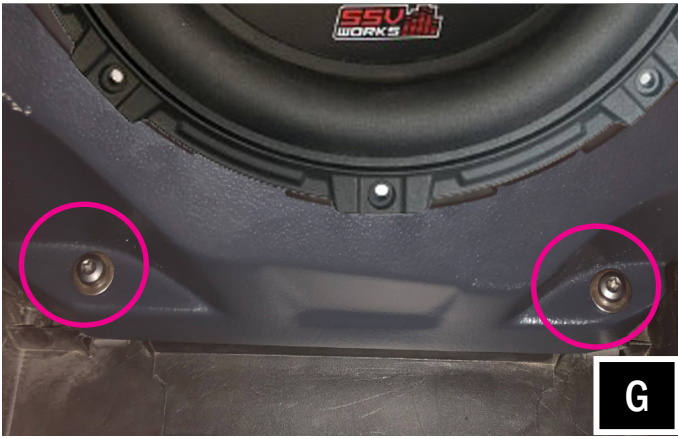
G. Secure the bottom of the enclosure with the provided M6x1.0x40mm T30 screws and washers to the M6 clip nuts attached to the firewall.
