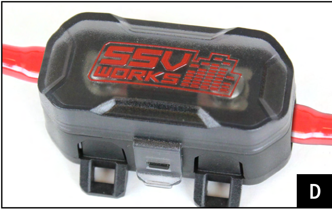
D. Remove the top of the fuse holder and extract the 2 screws. Insert the 40A fuse, screw the 2 screws back in and reattach the fuse holder top.
