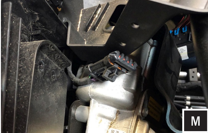
M. Locate the rear speaker output connector on the driver side of the dash cavity above the power steering motor. Remove the rear speaker output connector cap.
