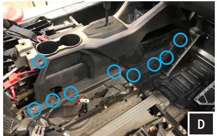
D. Remove the (1) push pin and (8) T40 screws from each side of the remainder of the center console.
