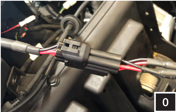
O. Connect the opposing end of the B-H2275 speaker harness to the door expansion speaker cable.
