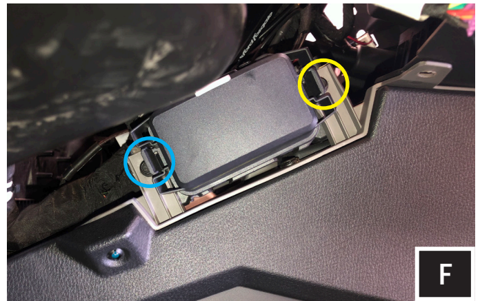
F. Loosen the 10mm screw on the left of the fuse block (circled in blue) and remove the 10mm screw on the right (circled in yellow). The fuse block is located on the driver side of the center console near the gas pedal.
