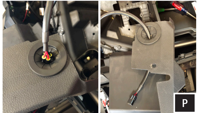
P. Route the door expansion speaker cable down the dash cavity and through the grommet on the front of the passenger console side panel.
