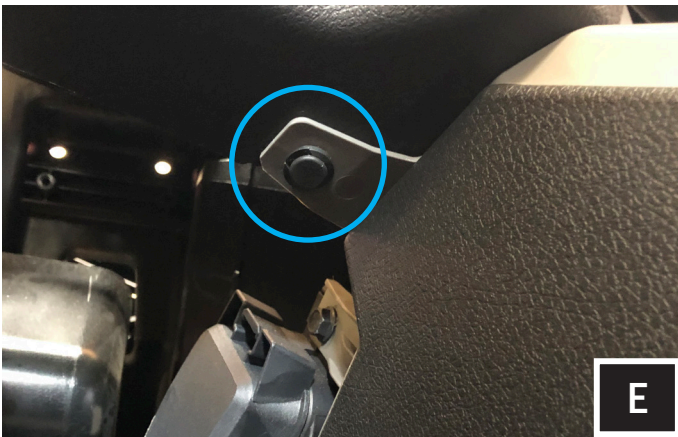
E. Remove the (2) push pins that are found on the bottom of the dash towards the center console.
