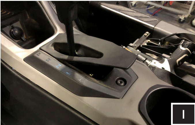
I. Lift the shift boot to expose the (1) T40 screw for removal
