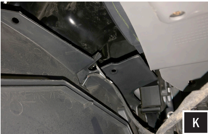
K. With the center console separated, unclip the LED from the driver and passenger console side panel. Once the LEDs have been unclipped, remove the driver console side panel from the vehicle.
