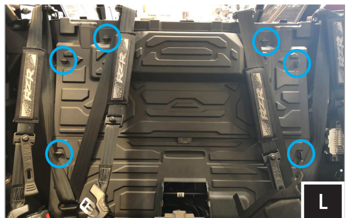
L. Twist the lock knobs on the rear firewall and remove the firewall.
