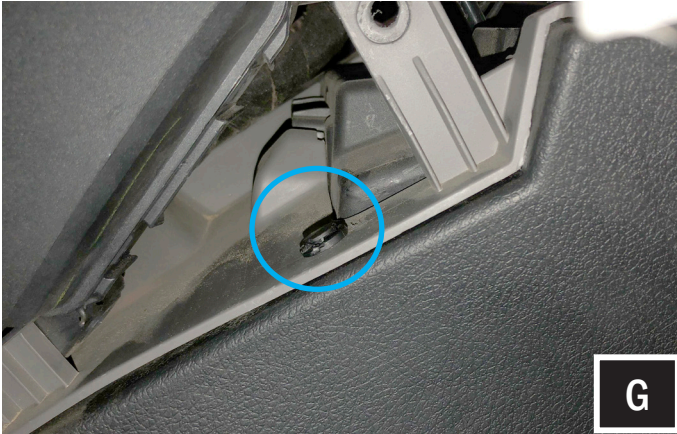
G. Rotate the fuse block counterclockwise and remove the now exposed push pin.
