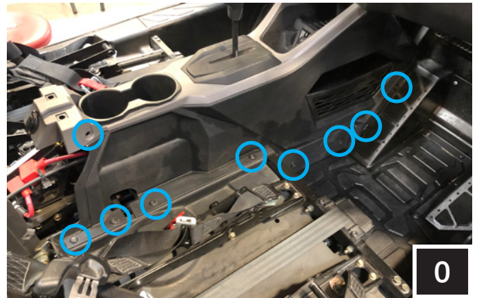
O. Remove the (1) push pin and (8) T40 screws from each side of the remainder of the center console.
