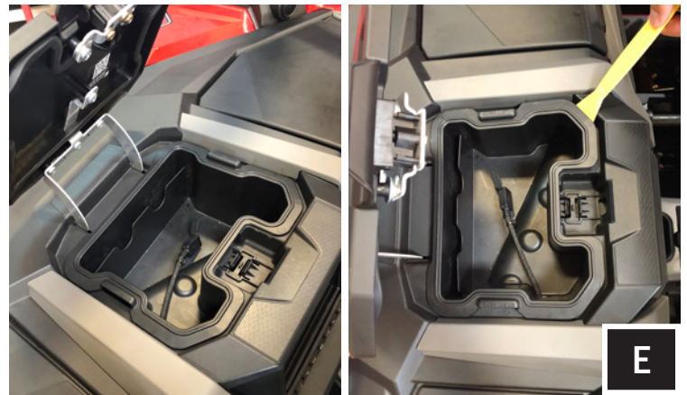
E. Open the top-center dash compartment and lift to remove the compartment tray. We recommend using a panel tool to assist releasing the tray from the compartment. Once the tray is separated from the compartment, pull out the USB cable from the tray, set tray to the side.
