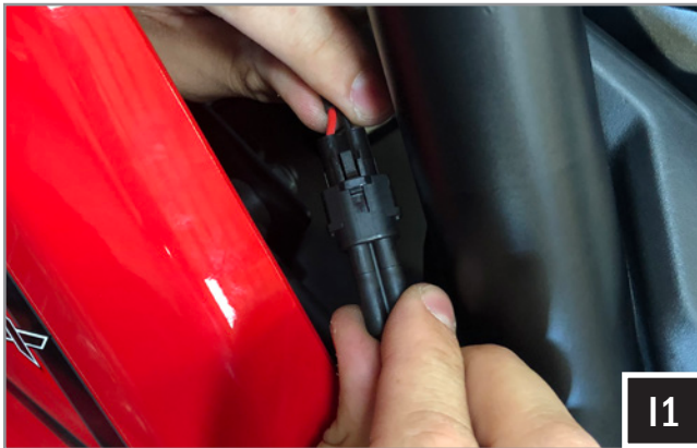
I1. Connect the speaker pods to the B-H2195 speaker harness.
