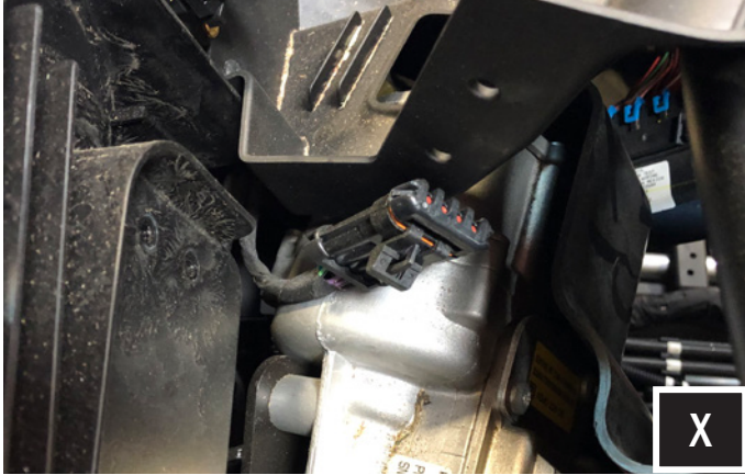
X. Remove the rear speaker output connector plug. The rear speaker output is located on the driver side of the dash cavity above the power steering motor.
