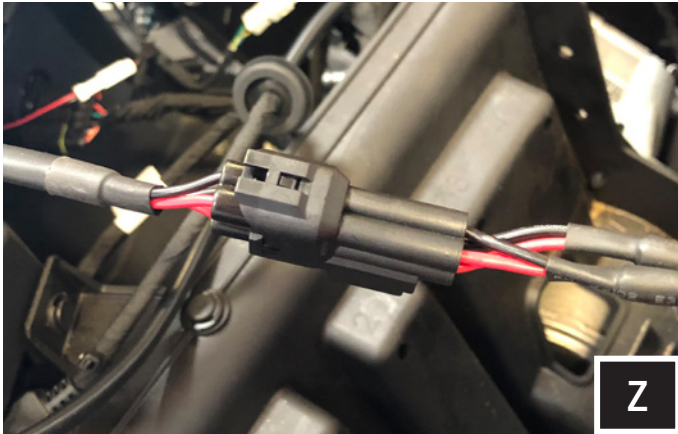
Z. Connect the opposing end of the B-H2275 speaker harness to the B-H1913 speaker extension harness.
