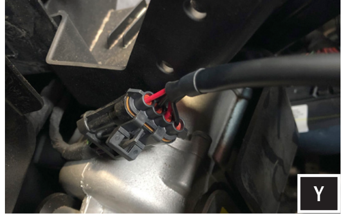
Y. Connect the B-H2275 to the factory rear speaker output.
