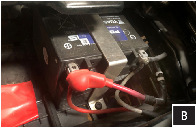
B. Using a 8mm wrench. Disconnect the negative battery cable from the battery.
