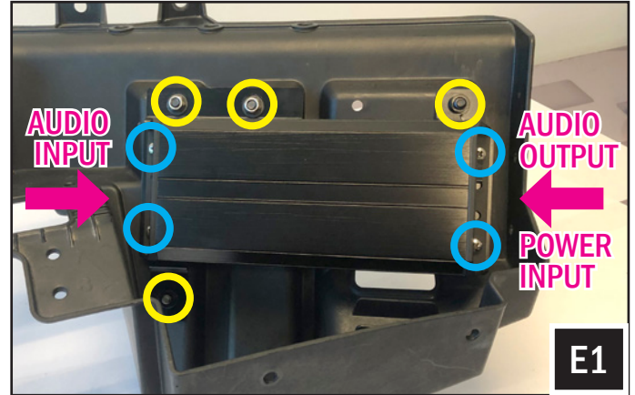
E1. Secure the 500.1 amp plate to the plastic tray with (4) T30 M6 screws washers and (2) 10mm lock nuts (circled in yellow). Fasten the 500.1 amp to the amp plate with (4) M4 screws (circled in blue).
