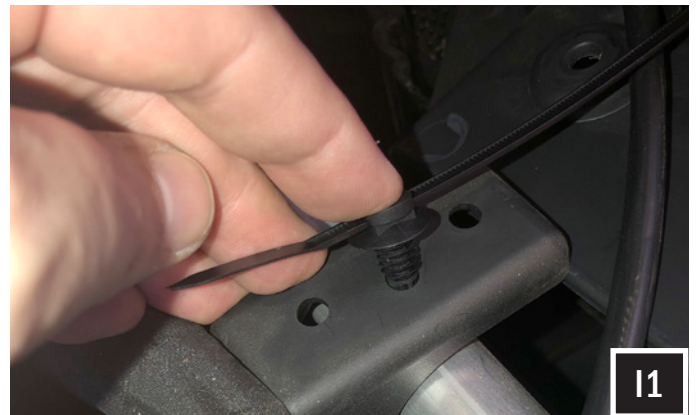
I1. Press zip-tie post into the zip-tie post holes that follow down the center of the vehicle. Starting from the rear of the vehicle, zip-tie the speaker cable to the vehicle and zip-tie post that were pressed in down the center of the vehicle in the previous step. Coil and zip-tie any slack in the harness towards the front of the vehicle.
