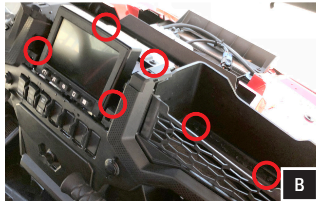
B. Extract the (4) T40 screws surrounding the ride command system and (2) push pins found in the dash pocket. *for non-ride command vehicles, less hardware may need to be removed for this step.
