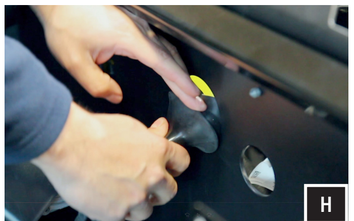
H. Unwrap the tape and pull the rubber wire grommet out of the firewall.
