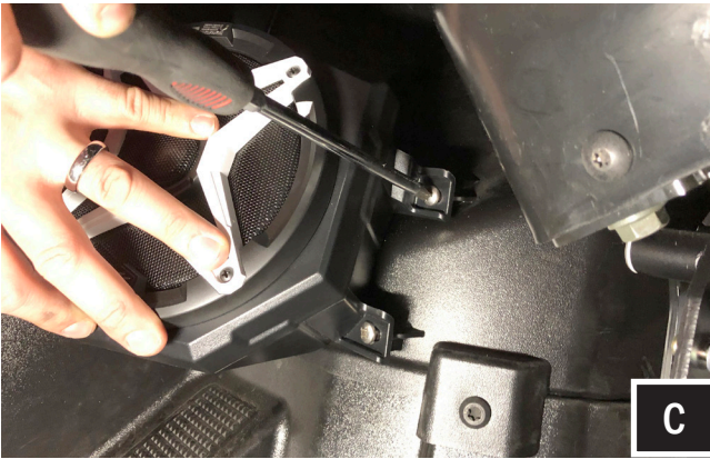
C. Using (2) #14 screw loosely secure the kick pod to the factory screw bosses.
