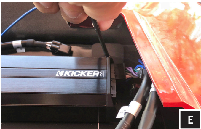
E. With the correct location marked, uninstall the amp tray and use a 13/64" drill bit to drill your pilot hole. With your pilot hole drilled, reinstall the amp tray. Use the self-tapping screw in the drilled hole location.
