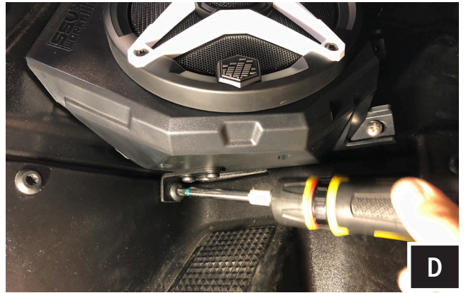
D. Re-use the factory T40 torx screw previously removed in Step A to loosely bolt through the lower kick pod bracket to vehicle panel. Once all three screws are in place go back and re-tighten.
