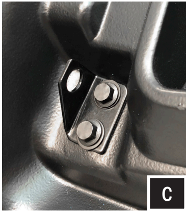
C. Install left and right door hinge brackets using (2) 8mm screws and washers for each side.
