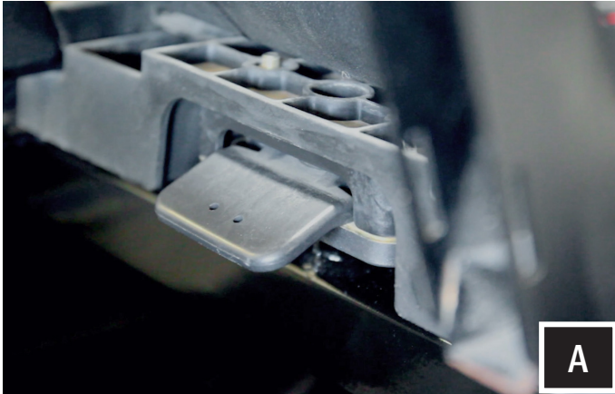
A. For ease of installation, remove all seats by releasing the handle behind each seat, push forward slightly while lifting up.
