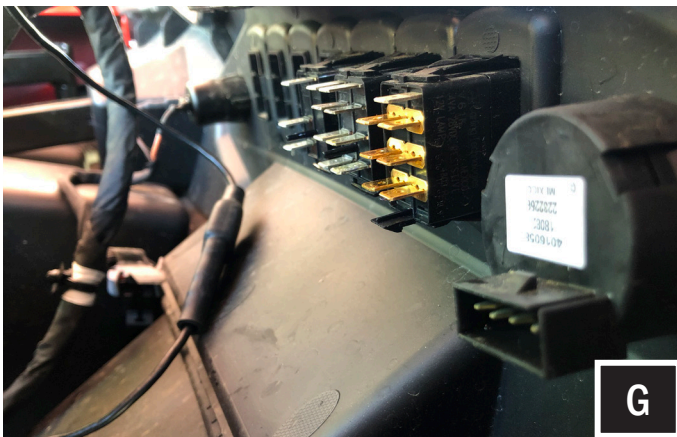
G. Label / take photos of the harnesses connected to the dash. Once recorded, disconnect harnesses, and remove dash.
