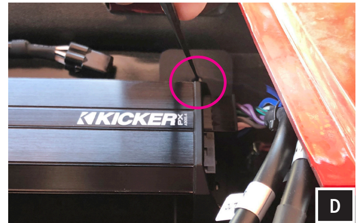
D. Using a scribe or punch, mark the location of the needed pilot hole on the passenger side of the tray.
