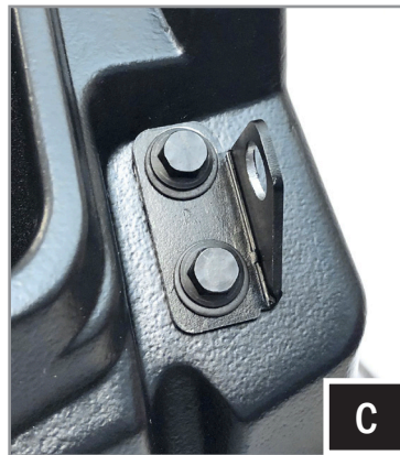
C. Install left and right door hinge brackets using (2) 8mm screws and washers for each side.
