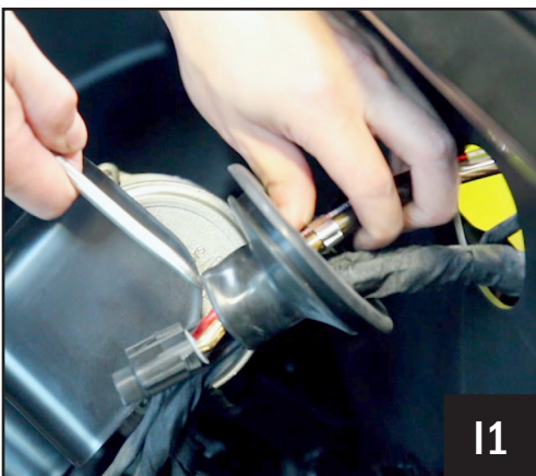
I. Starting from under the hood compartment, feed the connector of the power wire and B-H1151 rear harness female connector through the grommet into the dash cavity. In order to connect to the amplifier in a later step, pull about 18" of the amp power wire and B-H1151 into the dash cavity (I1). Route the additional length of the (ring terminal end) power/ground wire and B-H1151 down the exterior of the firewall along the factory wiring (I2). Pull the power/ground wire through to the center of the vehicle to the battery compartment. DO NOT CONNECT TO THE BATTERY (I3). B-H1151 will be used later for the cage mount speakers installation.
