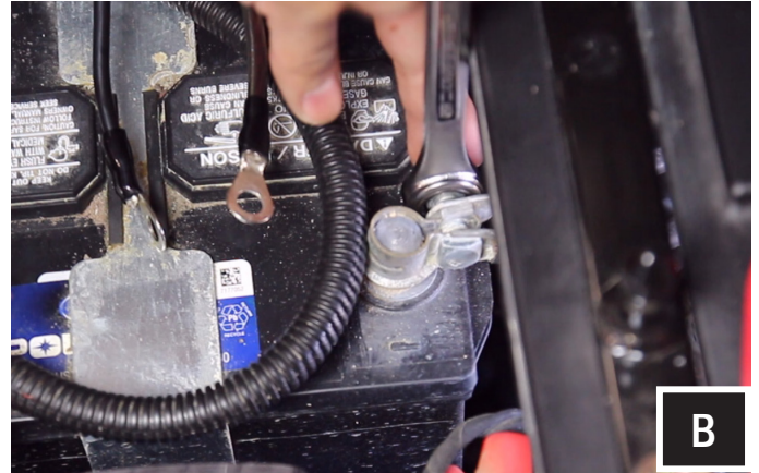
B. Disconnect the negative battery cable from the battery.
