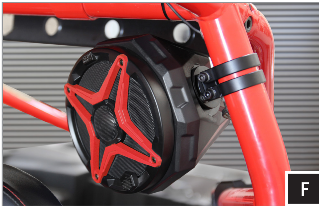
F. Route the speaker wire away from any moving parts and any sharp metal, then connect to the amplifier
