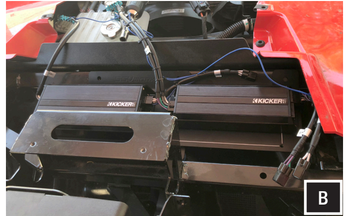
B. Place the amp tray into the mounting location by lining up the amp plate screw holes to the factory holes on the chassis.
