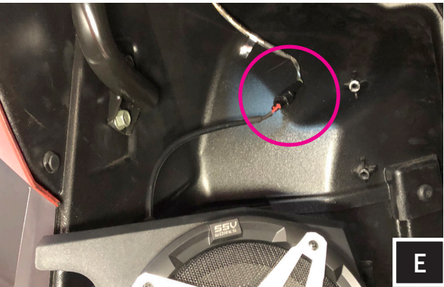
E. Connect the B-H1149 cable to the speaker pod and zip tie all cables to the frame.
