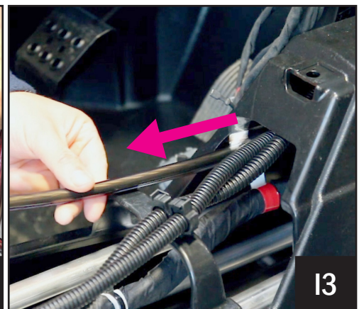
I. Starting from under the hood compartment, feed the connector of the power wire and B-H1151 rear harness female connector through the grommet into the dash cavity. In order to connect to the amplifier in a later step, pull about 18" of the amp power wire and B-H1151 into the dash cavity (I1). Route the additional length of the (ring terminal end) power/ground wire and B-H1151 down the exterior of the firewall along the factory wiring (I2). Pull the power/ground wire through to the center of the vehicle to the battery compartment. DO NOT CONNECT TO THE BATTERY (I3). B-H1151 will be used later for the cage mount speakers installation.
