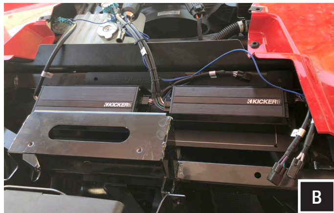
B. Place the amp tray into the mounting location by lining up the amp plate screw holes to the factory holes on the chassis.
