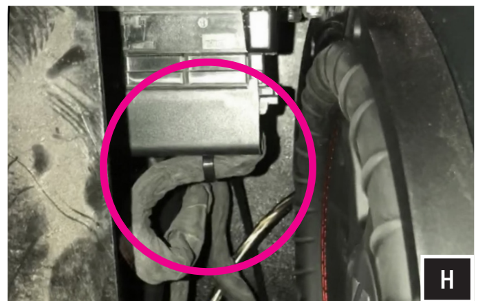
H. Cinch down zip tie as show in figure (H). Put the Dynamix brain tray back in place but DO NOT REINSTALL THE BOLTS.
