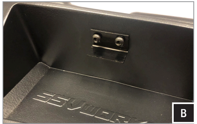
B. Install door latch onto enclosure with the provided (2) T30 M6x8mm screws.
