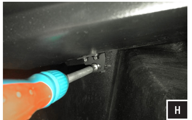
H. Fasten the provided #14 screw to secure the enclosure lower mounting bracket.
