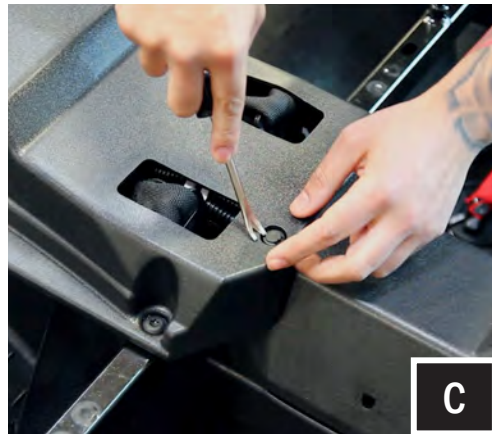
C. Remove all of the center console push pins and T-40 Torx screws. For 4-seat models, disconnect the harness attached to the 12v accessory socket.
