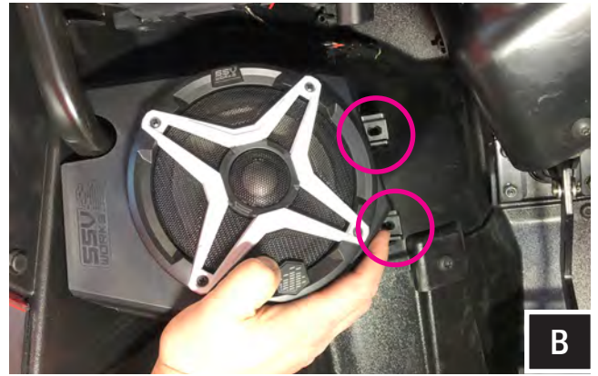
B. Place the driver kick pod into location so that both vehicle screw bosses line up with kick pod brackets.
