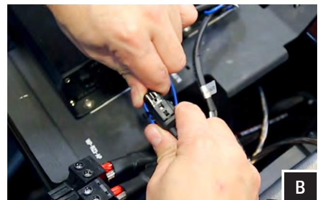
B. Connect the sub enclosure to the 800.5 amplifier output (sub)
