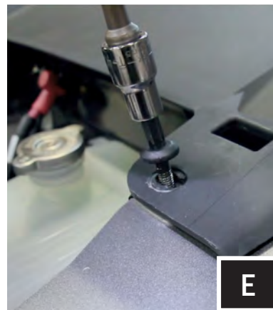
E. Remove center dash by unscrewing the (2) T-40 Torx screws and push center dash forward to unclip.
