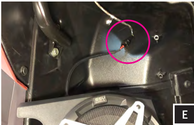
E. Connect the B-H1909 cable to both passenger and driver side speaker pods and zip tie all cables to the frame.
