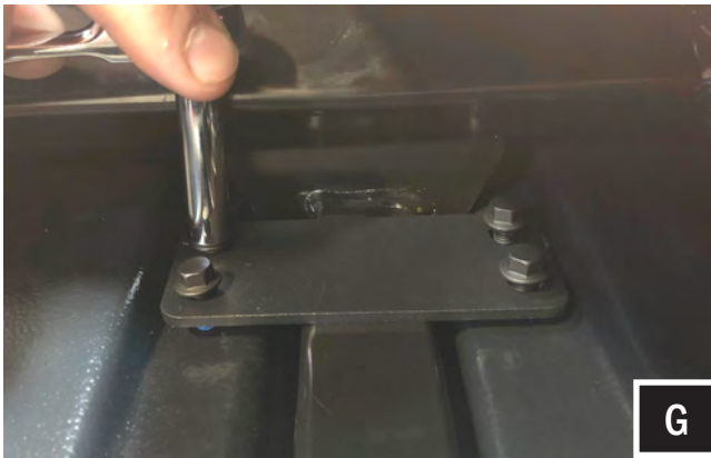
G. Place Bracket "A" into place towards the firewall, and fasten it into place with the (4) 8mm socket head screws and washers provided with the kit.
