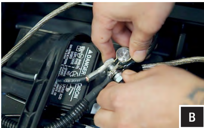
B. Unscrew the factory nut on the negative battery terminal. Install the 2 ground cables to the screw on the ground battery terminal. Re-install the factory nut.
