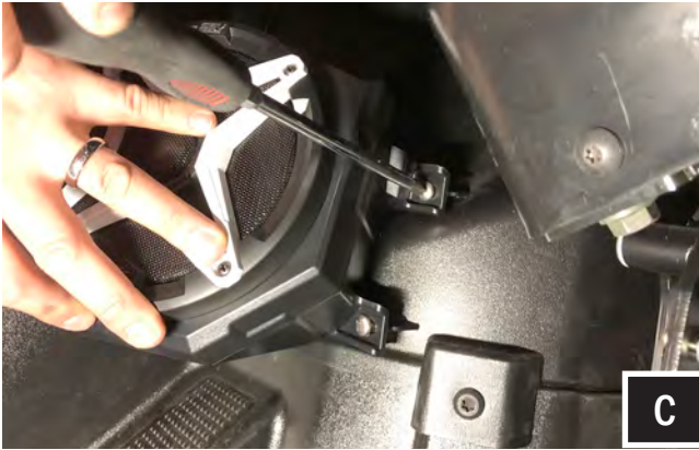
C. Using (x2) #14 screw loosely secure the kick pod to the factory screw bosses.
