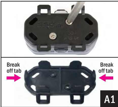
A1. Remove the bottom cover of the fuse holder by extracting the 2 screws. Break off the right and left side tabs on the bottom cover.
