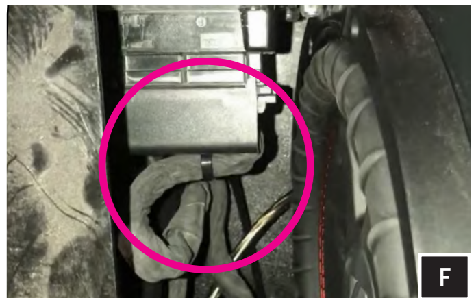
F. Cinch down zip tie as show in figure (F). Put the Dynamix brain tray back in place but DO NOT REINSTALL THE BOLTS.
