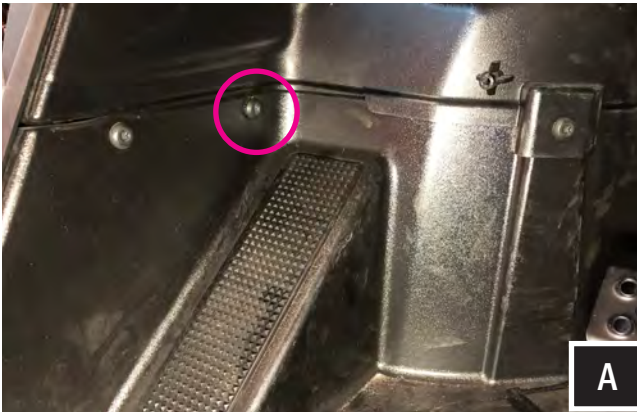
A. Starting at driver side footwell, remove the factory T40 torx screw as shown. Save this screw for Step D.
