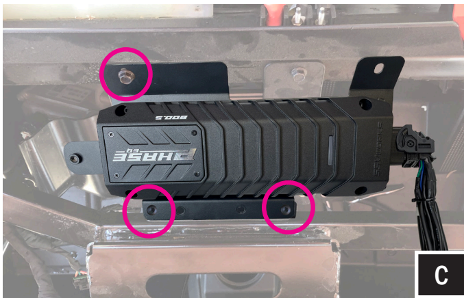
C. Secure the amp tray by using the 10mm factory bolt at the top, and two (2) T-30 torx bolts at the bottom mounting locations.
