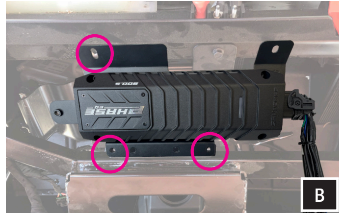
B. Place the amp tray into the mounting location by lining up the amp plate screw holes to the factory holes on the chassis and base bracket.
