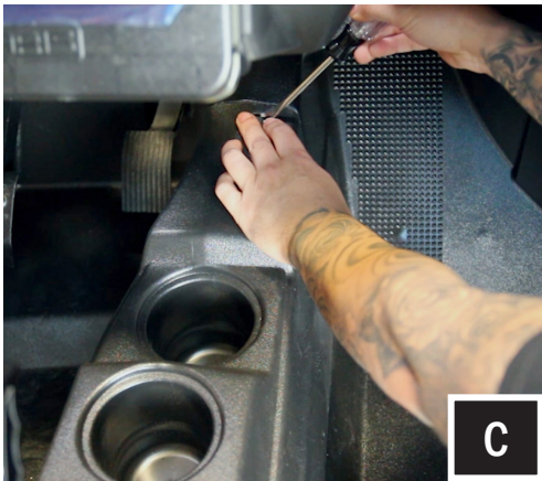
C. Remove all of the center console push pins and T-40 Torx screws. For 4-seat models, disconnect the harness attached to the 12v accessory socket.
