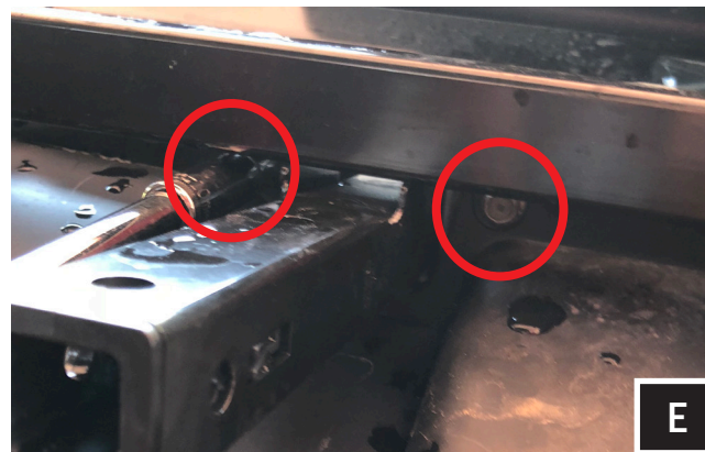
E. With the dash removed, extract the (2) 10mm bolts retaining the glovebox and remove the glovebox.
