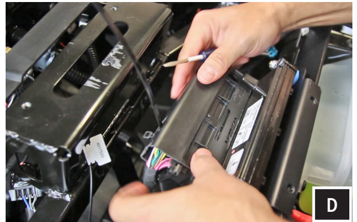
D. Snap the connector housing back into place over the connector.
