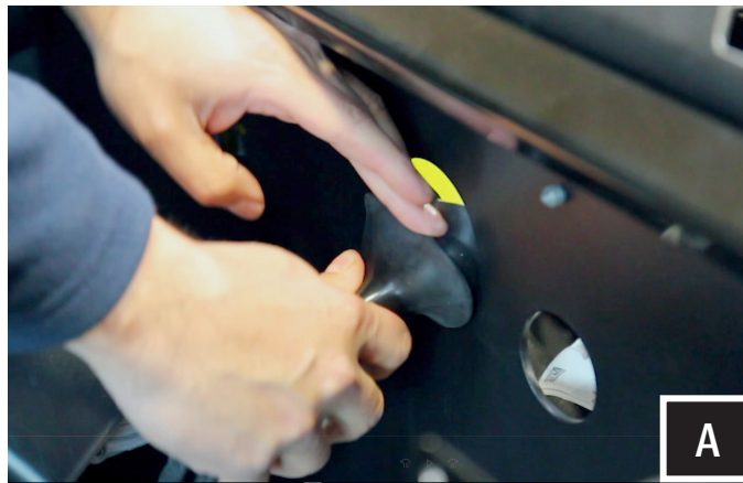
A. Unwrap the tape and pull the rubber wire grommet out of the firewall.
