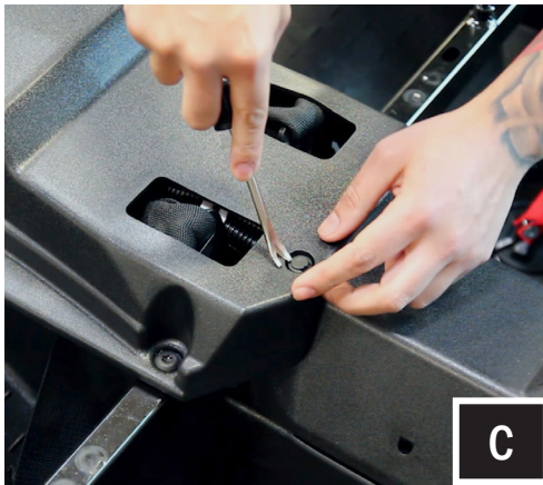
C. Remove all of the center console push pins and T-40 Torx screws. For 4-seat models, disconnect the harness attached to the 12v accessory socket.
