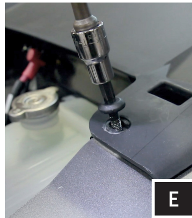
E. Remove center dash by unscrewing the (2) T-40 Torx screws and push center dash forward to unclip.
