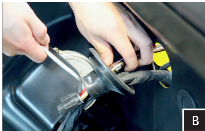
B. Starting from under the hood compartment, feed the connector of the power wire through the grommet into the dash cavity. In order to connect to the amplifier in a later step, pull about 18" of the amp power wire into the dash cavity.
