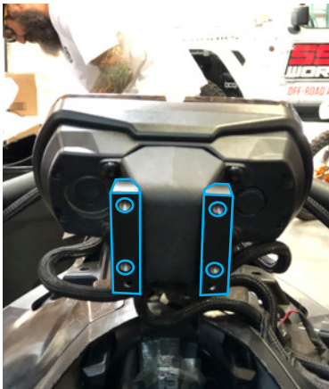
I. Align the RKR-2K over the mounting bases. Fasten the RKR-2K to the mounting brackets with the provided (4) M6x1.0x12mm torx screws and (4) M6 washers using a T30 Torx driver.
