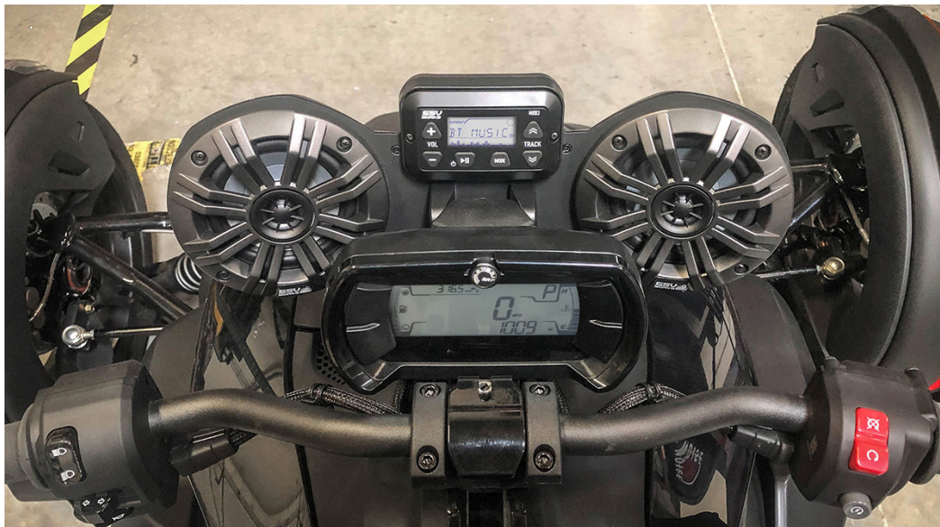
B1. Support the top of the center cover of the system and fasten the (2) #4 coarse threaded screws into the unit to complete cover installation. Test the system prior to reassembly of the vehicle.
