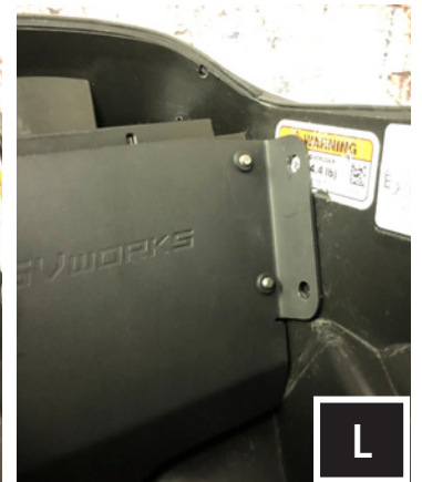
L. Seat the MRB3 brain assembly into the storage container. Verify that it is not pinching any of its harness'. MRB3 brain will make contact with the top of the compartment. Mark with a scribe or permanent marker the mounting points of the MRB3 bracket.
