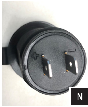
S. Connect the factory USB port to the power ground. Reference the back of the USB port to identify which terminal is power or ground.
