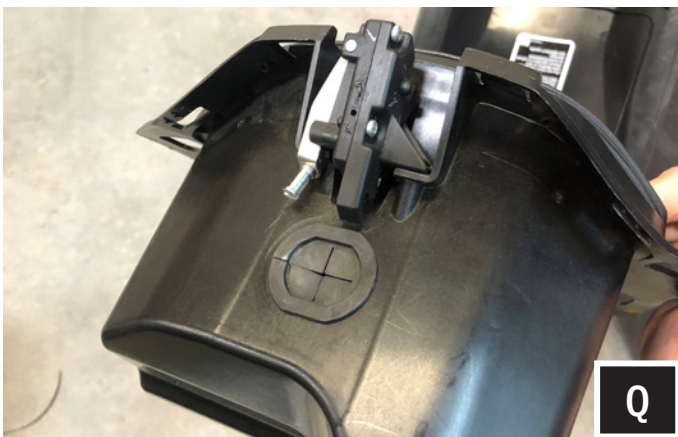
Q. Seat the cable grommet into the former location of the factory USB port.
