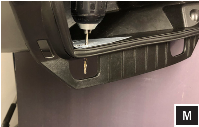
M. Remove the MRB3 brain assembly from the storage container and drill a pilot hole with a 1/8" drill bit at each marked point. Open up each pilot hole with a 5/16" drill bit.
