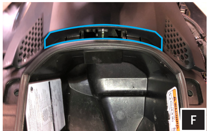
F. Using a panel tool, release the clips for the trim panel from the storage compartment.
