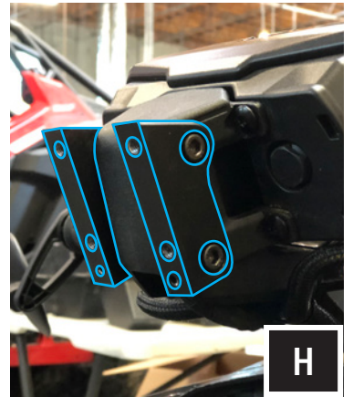
H. Fasten the RKR-2K mounting brackets to the front of the gauge cluster mount. With (2) 5mm allen screws on each side. Note the orientation of the mounting bases.
