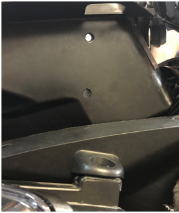
Y. From the exterior of the storage compartment, place (2) push pins on each side to mount the MRB3 in place.
