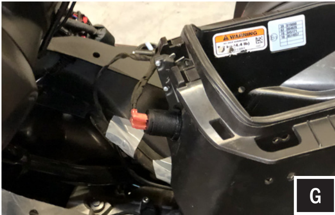
G. Once the fairing panel has been released, lift the front storage compartment and disconnect the USB charging port. Set the compartment aside for future steps.
