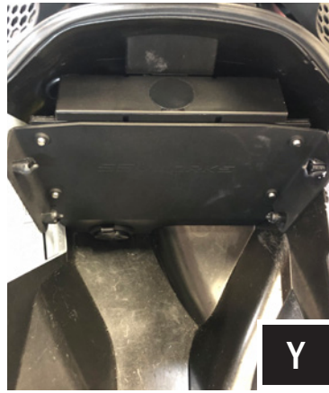
Y. From the exterior of the storage compartment, place (2) push pins on each side to mount the MRB3 in place.
