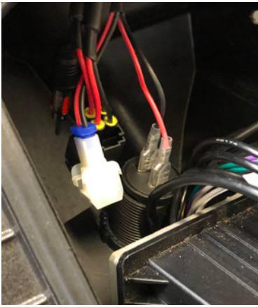
S. Connect the factory USB port to the power ground. Reference the back of the USB port to identify which terminal is power or ground.
