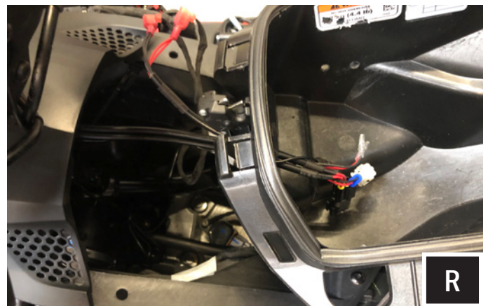
R. Route the RKR-2K cables into the storage compartment through the grommet.
