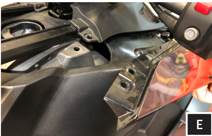
E. Pull the driver and passenger side panels off the Ryker.
