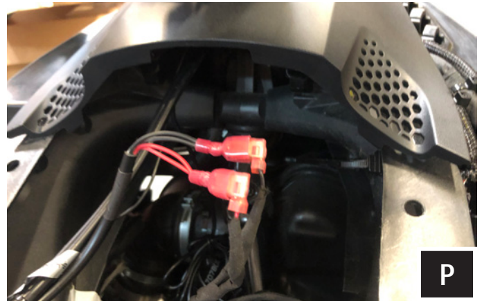
P. Connect the RKR-2K spade connectors to the factory power and ground that were disconnected from the factory USB port in Step G.
