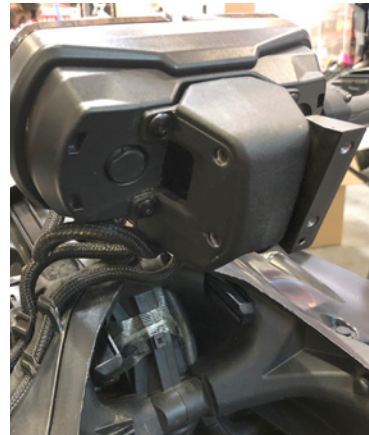
H. Fasten the RKR-2K mounting brackets to the front of the gauge cluster mount. With (2) 5mm allen screws on each side. Note the orientation of the mounting bases.
