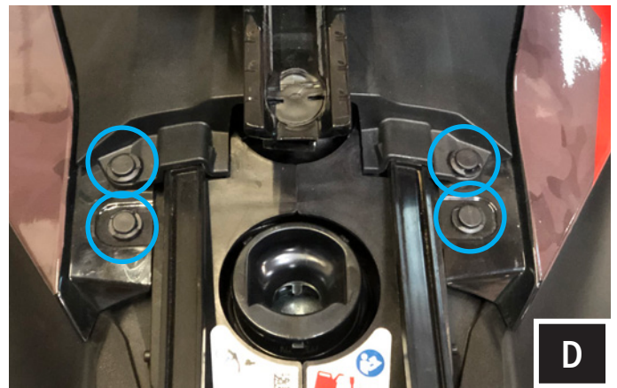
D. Slide back the fuel door. Remove the (4) push pins that are now exposed.
