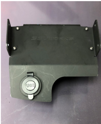
K. Place the USB charging port into the front of the MRB3 mounting plate and refasten the nut.
