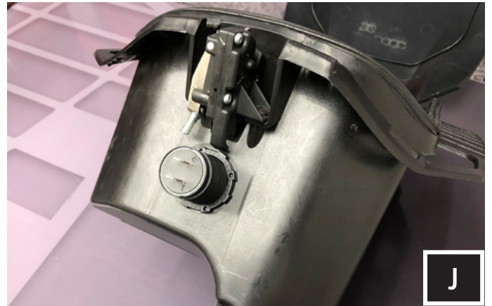
J. Unscrew the nut from the USB charging port and remove the charging port.
