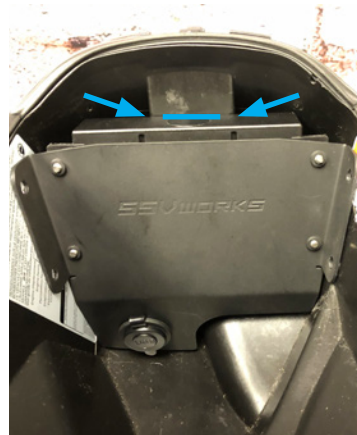
L. Seat the MRB3 brain assembly into the storage container. Verify that it is not pinching any of its harness'. MRB3 brain will make contact with the top of the compartment. Mark with a scribe or permanent marker the mounting points of the MRB3 bracket.
