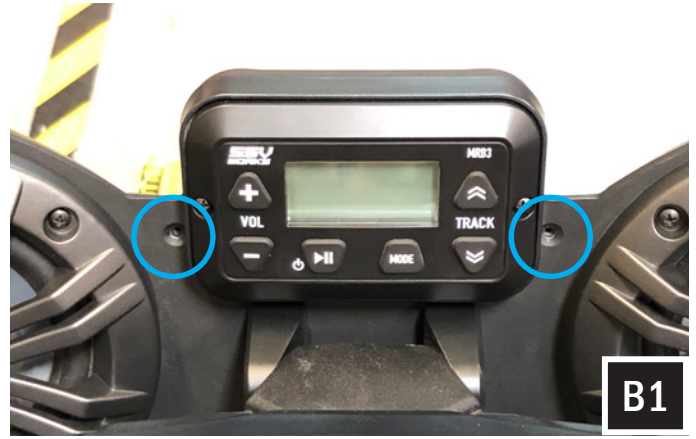
B1. Support the top of the center cover of the system and fasten the (2) #4 coarse threaded screws into the unit to complete cover installation. Test the system prior to reassembly of the vehicle.
