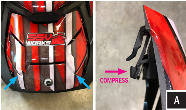
A. Compress the locking tabs to the hood and slide the hood down simultaneously to release the hood and remove.
