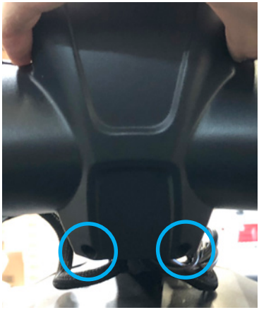
A1. Hold the center cover onto the front of the RKR-2K, fasten the (2) M3 machine screws into the system to retain the cover.
