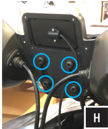
I. Align the RKR-2K over the mounting bases. Fasten the RKR-2K to the mounting brackets with the provided (4) M6x1.0x12mm torx screws and (4) M6 washers using a T30 Torx driver.
