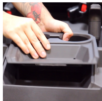
C. With push pins extracted, lift to remove the cup holder and gauge cluster.
