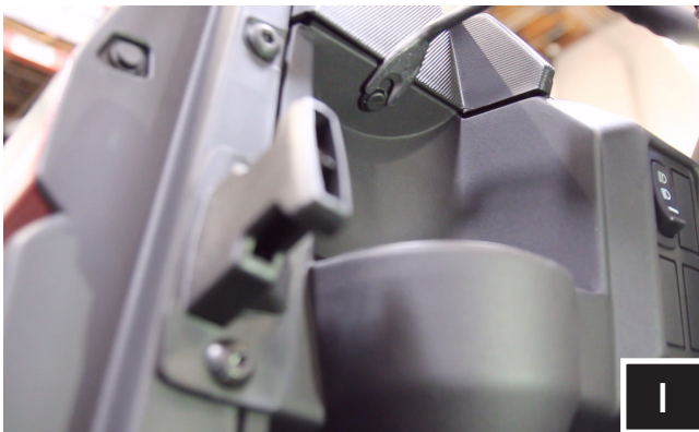
I. Extract push pins located above driver and passenger side cup holders.
