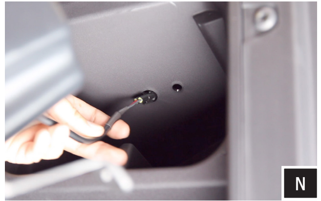
N. Located on the inside top of the pocket you will have two holes, route speaker wire through the larger hole. The smaller hole will be used to mount the pod in Step P.
