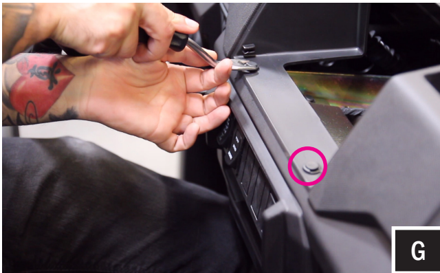
G. Extract push pins exposed from cup holder removal.
