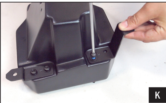
K. Using the supplied M6 screws and small washers, install the brackets to kick pods.
