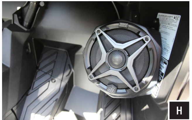
H. Route the speaker wire away from any moving parts and any sharp metal, then connect to the amplifier. Repeat installation on opposite side.
