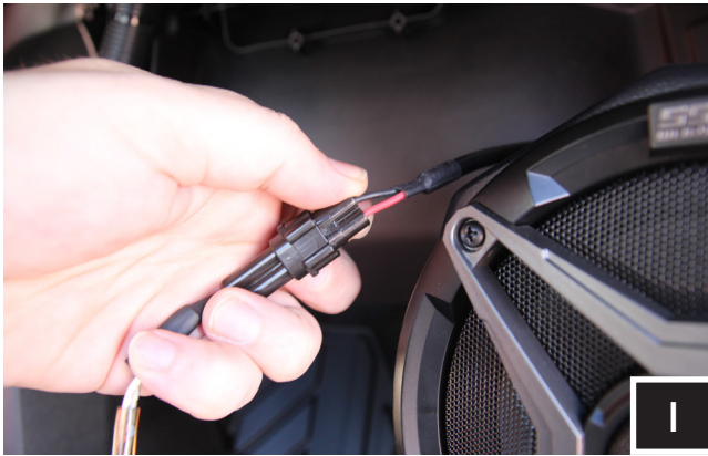
I. Connect the B-H1149 speaker wire outputs to each pod.
