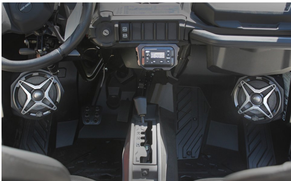
K4. Connect the Front Speaker output from the MRB3 brain to the B-H1149 speaker harness.
