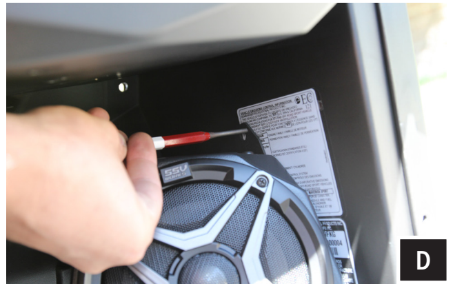
D. While holding the pod in place, use a scribe to mark a drill point for the pilot hole.
