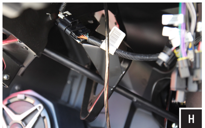
H. Route B-H1149 speaker harness along the underside of the dash. Avoid sharp edges and rotating parts, zip tie harness in place. Note: Verify each end of the harness goes to the correct side of the vehicle. Each connector is properly labeled driver/passenger
