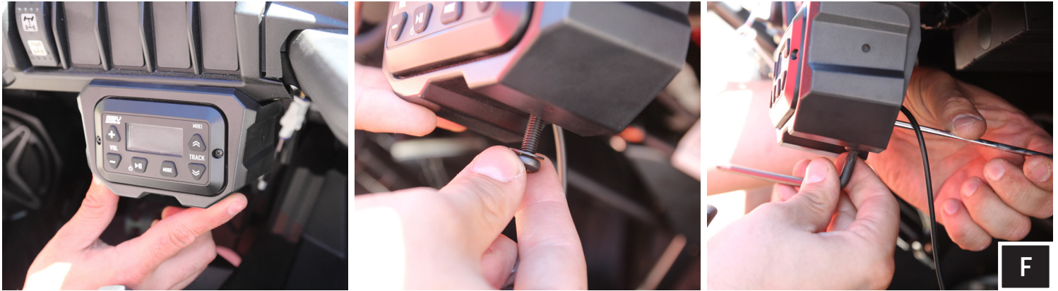
F. Put the assembled DM3 in place. Using the SSV provided hardware (T30 torx screw, washers, and 10mm nut) fasten down the DM3 from the bottom. Drilling for this step is not required, the hole needed is factory.
