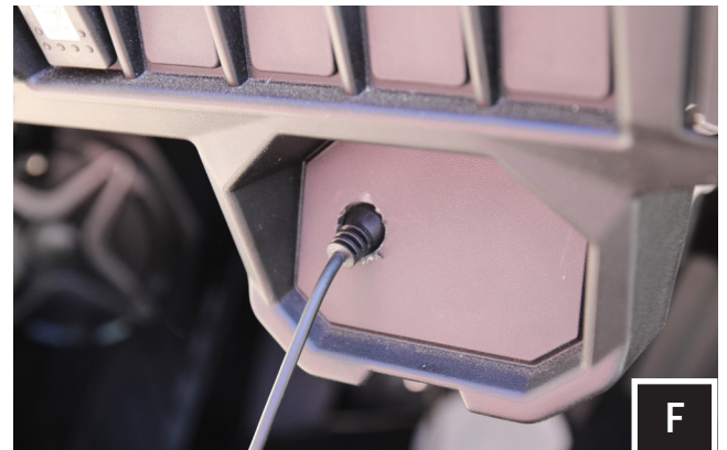
F. Feed controller cable through the 9/16" hole that was drilled in figure E.
