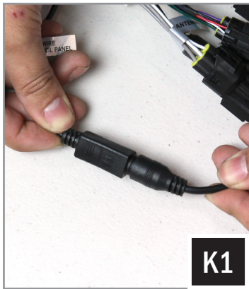
K1. Connect the MRB3 controller to the brain.
