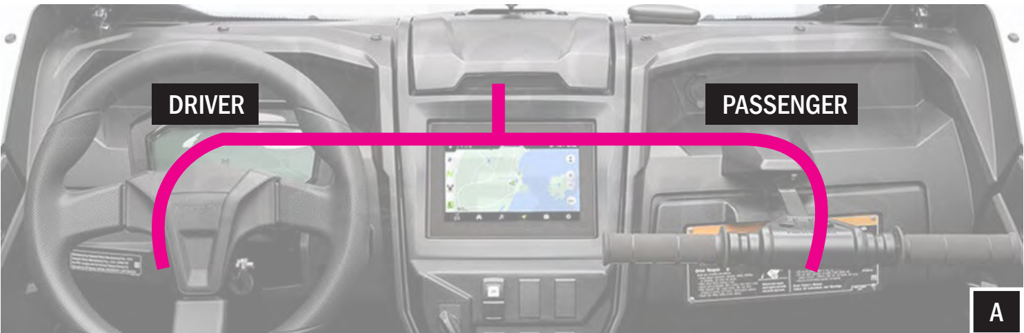
A. B-H1909 connects to Front Output on 800.5 Amp and splits off to plug into each pod
