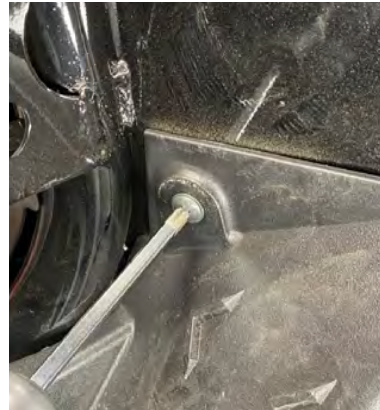
E. Starting on the drivers side, Remove the factory screw at the top of the footrest. Place the speaker pod in position and use the same factory screw to attach the bottom bracket.
