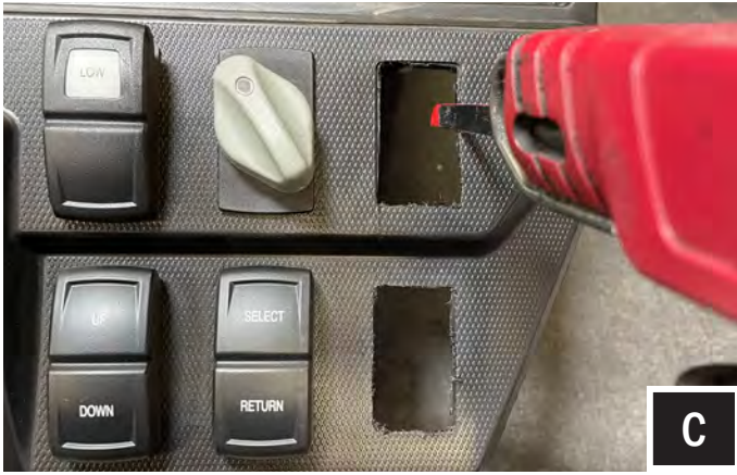
C. Using an air saw or dremel cut out holes on your rocker switch panel. Clean up with a file.
