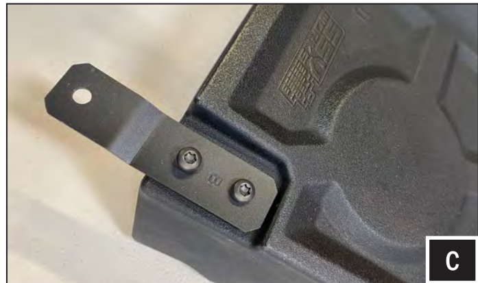
C. Attach Bracket "B" to the driver side pod and Bracket "F" to the passenger side pod as shown using two (2) M6 screws and washers.
