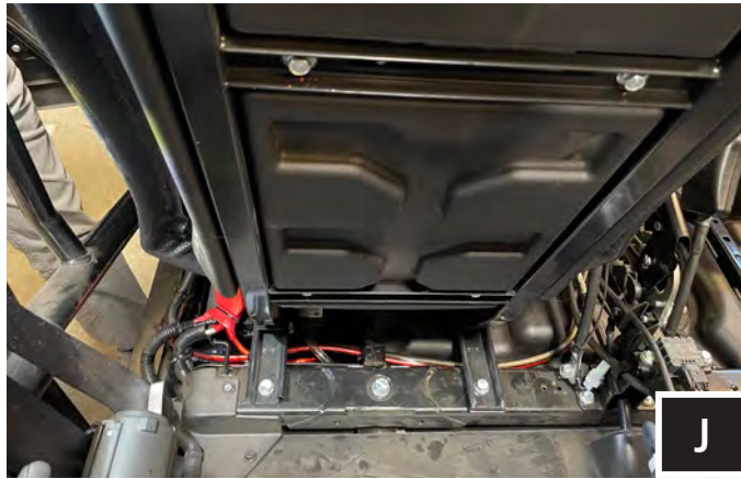
J. Run wires behind driver seat and make sure to keep away from any moving parts. Zip tie to factor harness. K. Connect to battery terminal.
