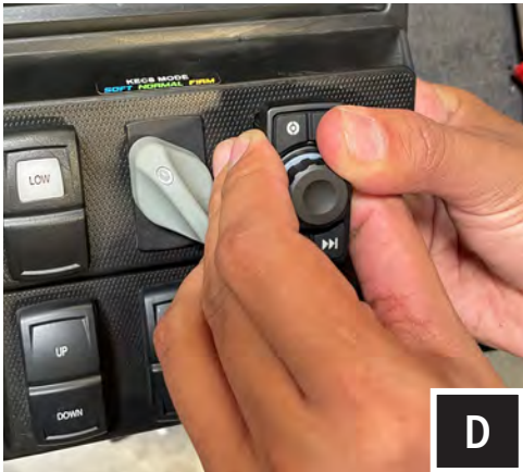
D. Push in both Rock and Ride switch and the MRB2R controller.
