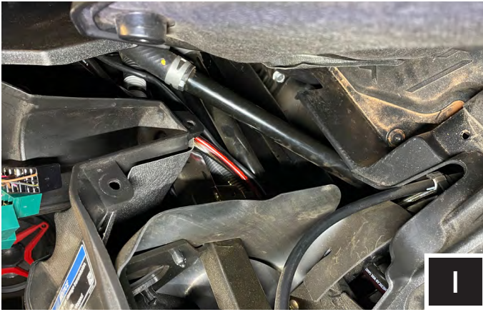
I. Once the seat, center console, and passenger side center console cover are removed, run wires back to battery.
