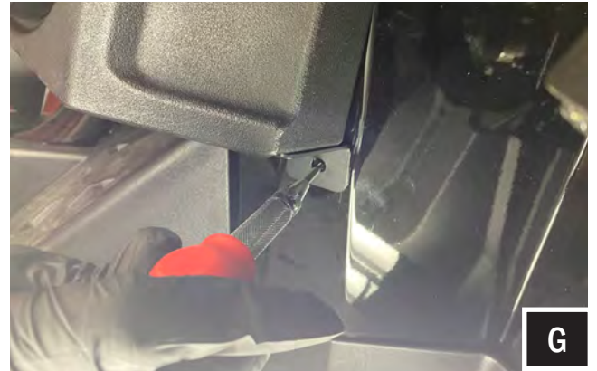
G. Using a punch tool, create a drill guide at the center of Bracket "C" hole.
