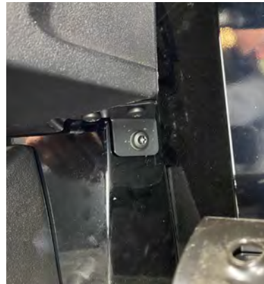
I. Connect Bracket "C" by pushing the 25mm M6 screw through the drilled hole and hand tighten the locking nut from the other side of the floorboard. It is recommended to have 2 people complete this step, one person on each end of the screw as it is tightened.
