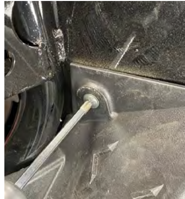
E. Starting on the drivers side, Remove the factory screw at the top of the footrest. Place the speaker pod in position and use the same factory screw to attach the bottom bracket.
