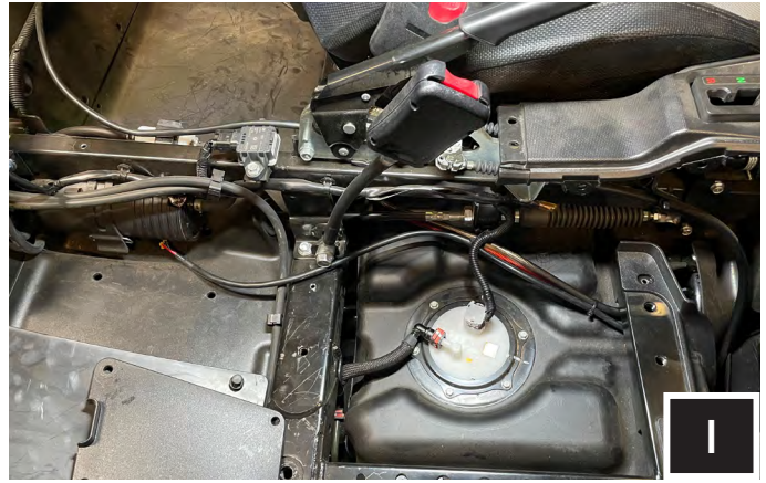
I. Once the seat, center console, and passenger side center console cover are removed, run wires back to battery.
