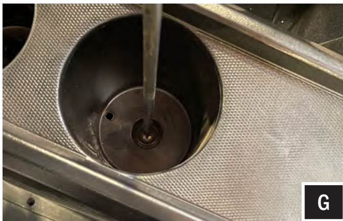
G. Remove Phillips screw inside cupholder.
