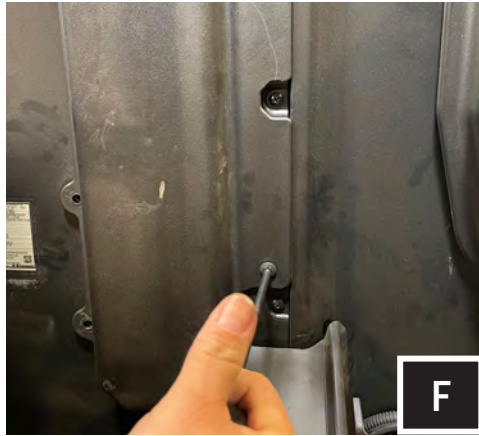
F. Remove phillips screws and panel clips to remove the center panel on the back wall.
