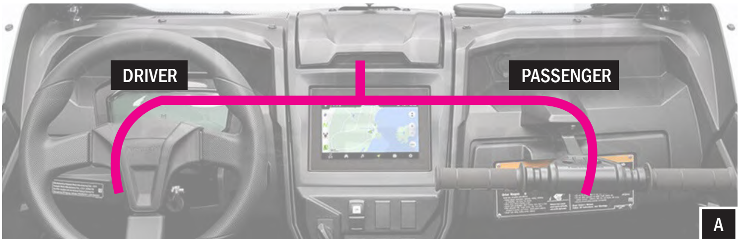
A. B-H1909 connects to Front Output on 800.5 Amp and splits off to plug into each pod
