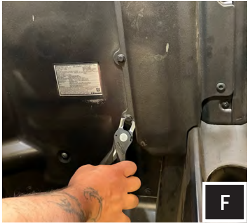
F. Remove phillips screws and panel clips to remove the center panel on the back wall.
