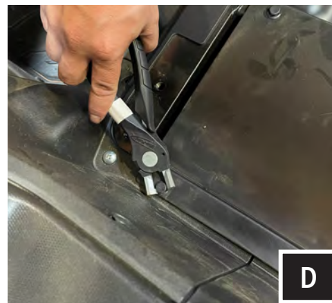
C. Remove panel clips from passenger side center console and pull panel out enough to access the insed for running cables. D. Using clip removal tool, unclip the (4) clips and remove fuel pump cover.
