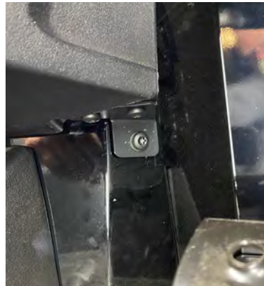
I. Connect Bracket "C" by pushing the 25mm M6 screw through the drilled hole and hand tighten the locking nut from the other side of the floorboard. It is recommended to have 2 people complete this step, one person on each end of the screw as it is tightened.
