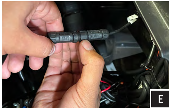
E. Carefully line up the plugs for Rock & Ride as well as for the MRB2R, push them together and hand screw nut to tighten.
