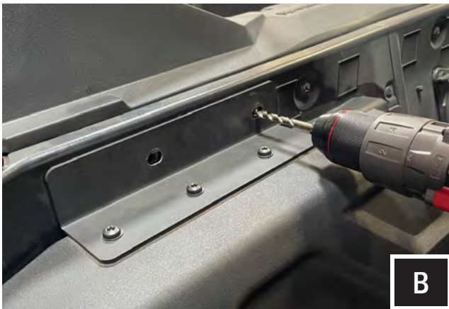
B. Place sub enclosure in its designed location behind passenger seat and using 9/32" or 17/64" drill bit, drill pilot holes where needed.
