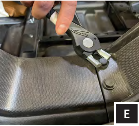
E. Remove clips and Phillips screws from the center console.
