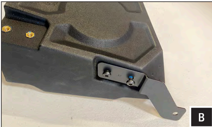
B. Attach Bracket "A" to the driver side pod and Bracket "E" to the passenger side pod as shown using two (2) M6 screws and washers.
