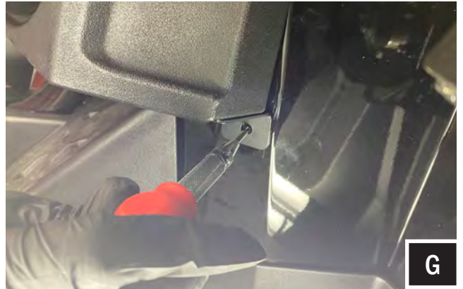
G. Using a punch tool, create a drill guide at the center of Bracket "C" hole.
