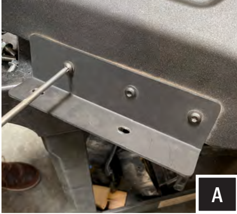
A. Mount plates to sub enclosure using the torx screws provided.
