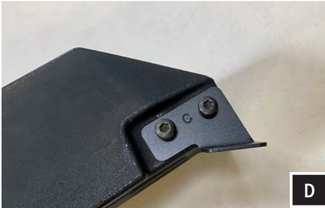
D. Attach Bracket "C" to the driver side pod and Bracket "G" to the passenger side pod as shown using two (2) M6 screws and washers.
