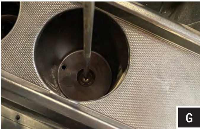
G. Remove Phillips screw inside cupholder.
