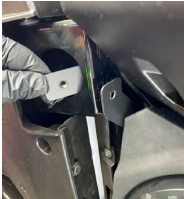
F. Place Bracket "D" through the door jam hole (as shown above) and use a M6 screw and washer to attach Bracket "A"
