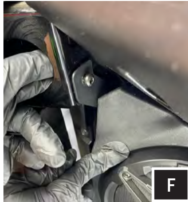
F. Place Bracket "D" through the door jam hole (as shown above) and use a M6 screw and washer to attach Bracket "A"
