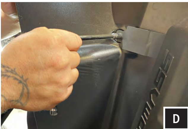
D. Place sub enclosure back in its designed location, place plastic spacer between sidewall of machine and side bracket. Tighten bolt down.
