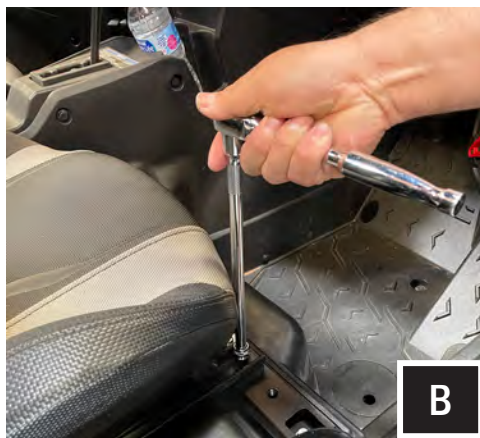
A. Run Power and Ground for Phase EQ from the amp to the center console. B. Remove the seat, use a 13mm socket and wrench to remove front (2) bolt and nut, and use a 18mm socket to remove (2) rear nuts and seat belt nut (repeat on other seat)
