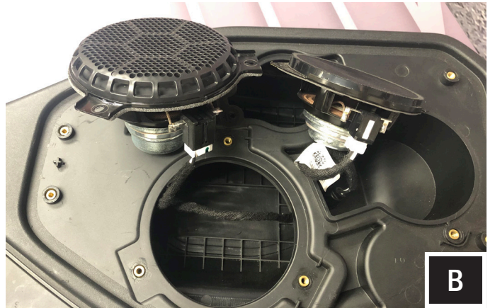
B. Remove the (4) T30 torx screws from the port and (5) T20 screws from both speakers. Pull out the port, disconnect and set the speakers aside.
