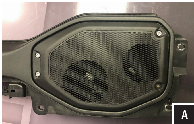
A. Remove the (4) 5mm allen head screws and grill.
