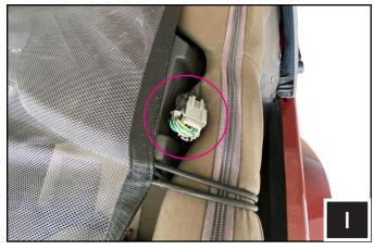
I. Hold the SSV soundbar up to the vehicle roll cage and connect to the factory plug.
