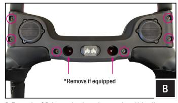
B. Extract the x6 Bolts securing the enclosure to the vehicle roll cage and set aside for use on the last step. If your vehicle is equipped with a top remove the two hand threaded cups along each side of the dome light. Remove the soundbar from the vehicle.
