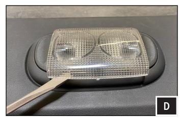
E. Using a panel removal tool or flat head screwdriver, unsnap the plastic dome light lens.
