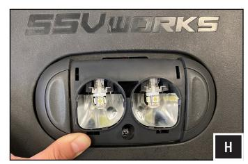
H. Hold down the domelight while fastening the provided SSV Works #2 Phillips screw to secure the dome light down to soundbar.
