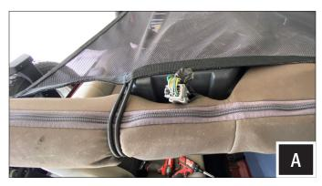
A. From the passenger side of the vehicle locate the connector at the top of the soundbar and disconnect.
