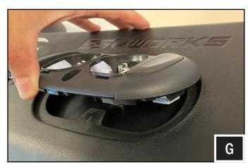
G. The SSV soundbar is made thicker than the factory soundbar to support the 8" speakers. The dome light will fit tight because of this. Angle in the dome light so both plastic tabs hook onto the material first then push in and lay flat.
