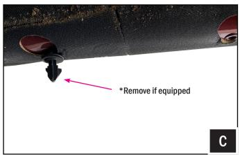
C. Once the factory soundbar has been removed use a panel removal tool and extract the plastic locating pin. These will not be needed for the new soundbar.
