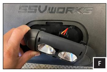
F. Connect the factory dome light into the SSV soundbar.
