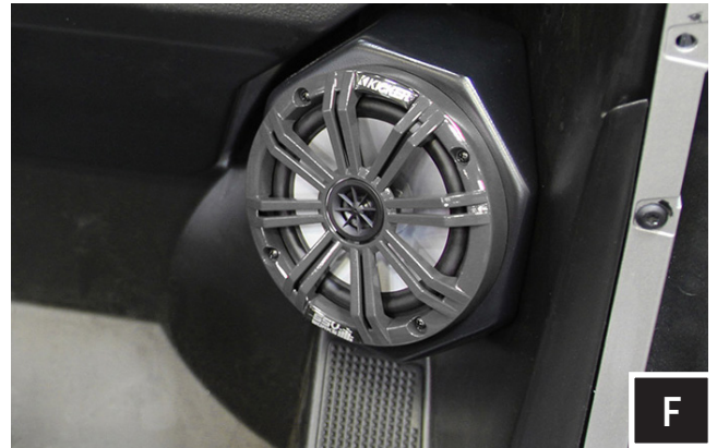
F. Route the speaker wire away from any moving parts and any sharp metal, then connect to the amplifier. Connecting the GN-F65 using the pre-installed, two-pin connector will require an optional SSV Works plug-&-play harness (WP-H1149 - sold separately). If you are not using the WP-H1149 harness, simply cut off the two-pin connector and follow the wiring instruction below.
