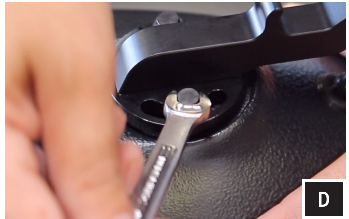
D. Tighten the 8mm bolts once you have the speaker pods in your desired location.
