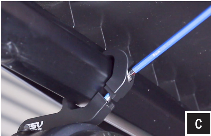
C. Using a T5 hex key tighten clamp until it secures to cage.
