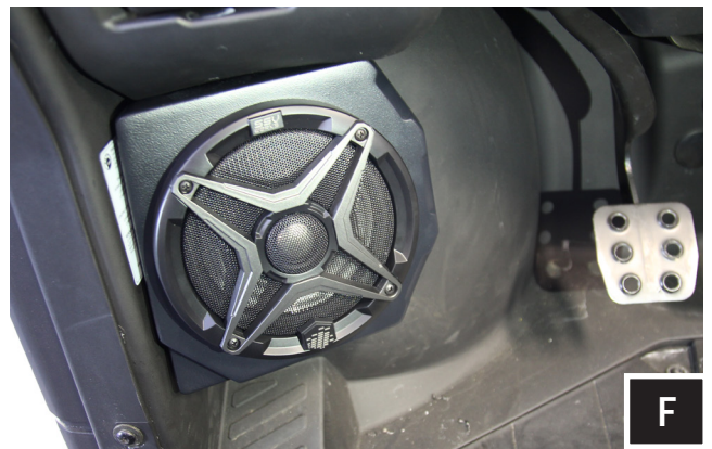
F. Route the speaker wire away from any moving parts and any sharp metal, then connect to the amplifier. Connecting the DF-F65 using the pre-installed, two-pin connector will require an optional SSV Works plug-&-play harness (WP-H1149 - sold separately). If you are not using the WP-H1149 harness, simply cut off the two-pin connector and follow the wiring instruction below.
