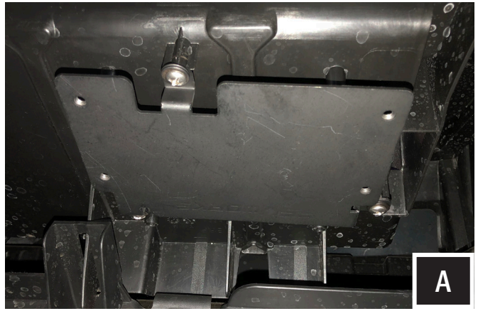
A. Using the (3) mounting bosses on the underside of the dash of the passenger side pocket, place the MRB3 brain tray on the bosses and fasten it into place with the provided (3) screws and washers.
