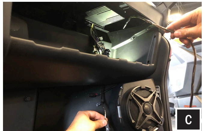
C. Route speaker harness B-H1149 across the inside of the dash to the driver and passenger side. Avoid any moving rotating parts. For the passenger side, tuck the harness down the side of the dash, and pull it through to connect to the pod.
