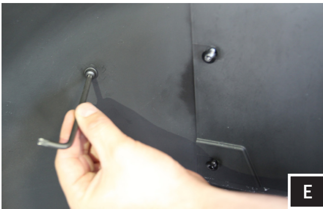
E. Place enclosure in location for mounting. Re-use the (2) factory T30 torx screws and SSV provided M6 screws and washers. to mount the pod loosely. Once all screws have been loosely installed, tighten down by hand.
