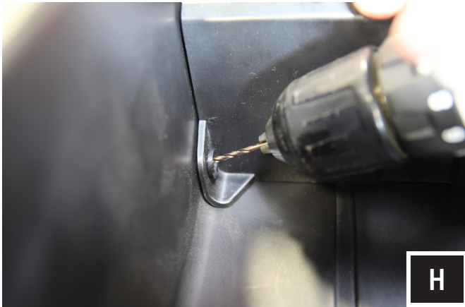
H. Drill pilot holes through the drill bit guides that were inserted into the back tabs in Step B with a 1/8" drill bit.
