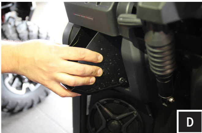
D. For ease of access to route the driver side of the harness remove the pocket located above the pod. To remove the pocket, pull the pocket open, slightly squeeze the sides, and twist it out. Connect to the driver side speaker pod.
