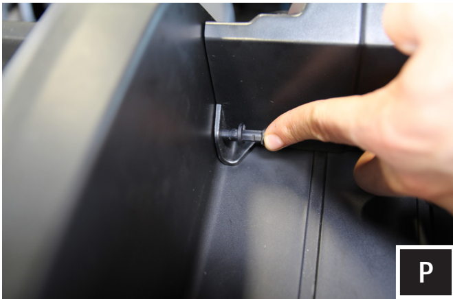
P. Insert push pins through the back of the DM3 into the dash.
