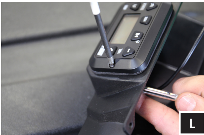
L. Feed the MRB3 cable through the controller opening and place the MRB3 controller in the DM3. Fasten down with the two (2) provided Phillips screw and 5.5mm nuts.
