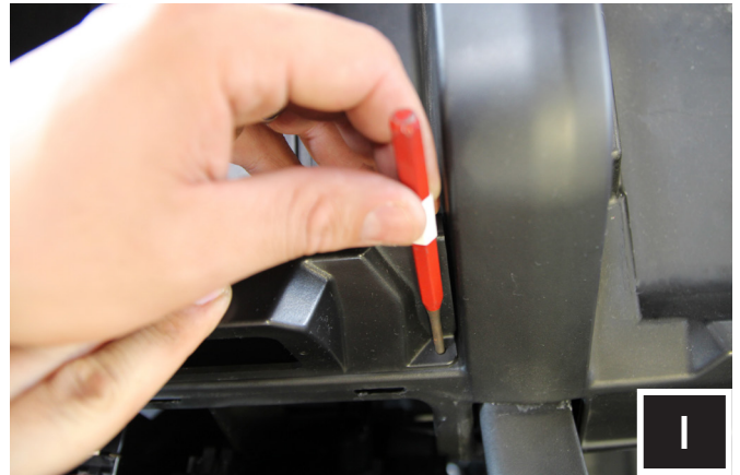
I. Place the MRB3 dash mount into its intended location and scribe marks through the front mounting tabs to drill pilot holes.
