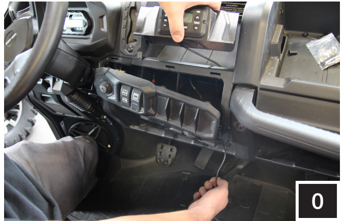
O. Route the MRB3 controller cable through the 9/16" hole drilled in Step C and set the DM3 into place
