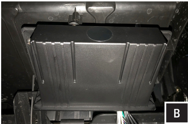
B. Once the MRB3 brain tray is secured, mount the MRB3 brain to the tray with the provided (4) M5 screws and washers.
