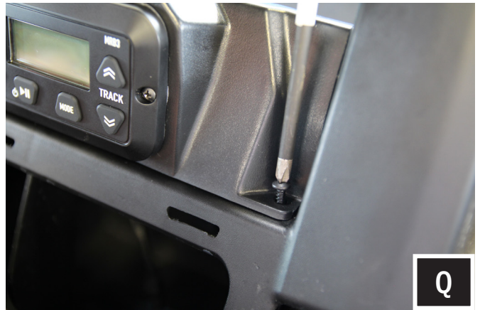
Q. Fasten the front of the DM3 with provided two (2) Phillips screws.
