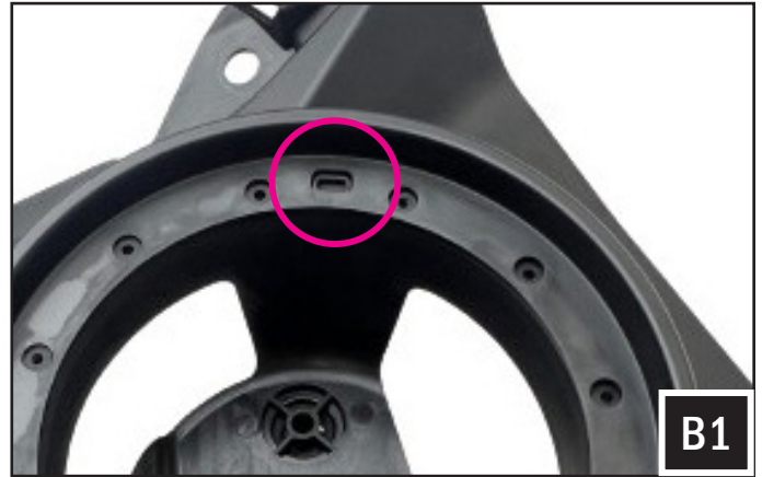
B. Line up the alignment peg of the speaker bucket to the oval hole on the Mav R speaker panel.
