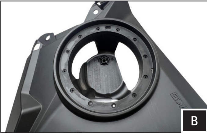
B. Hold the speaker bucket to the back side of the Mav R speaker panel.
