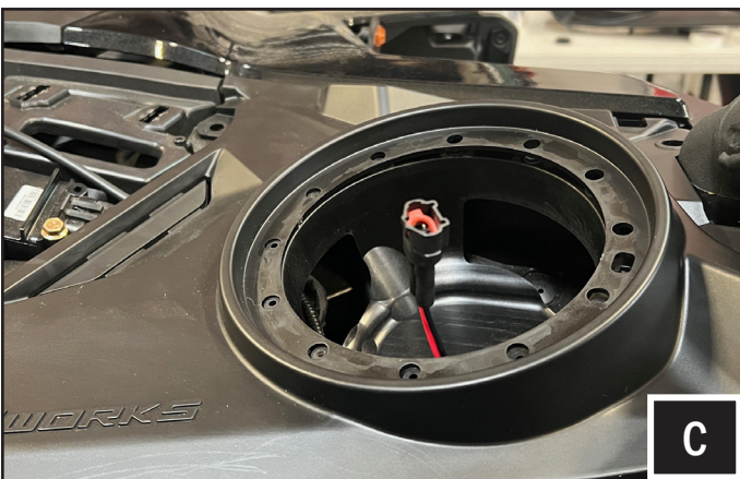
C. Put the panel on the dash and press in the bucket to the rubber grommet. Run the speaker wire to the speaker bucket.
