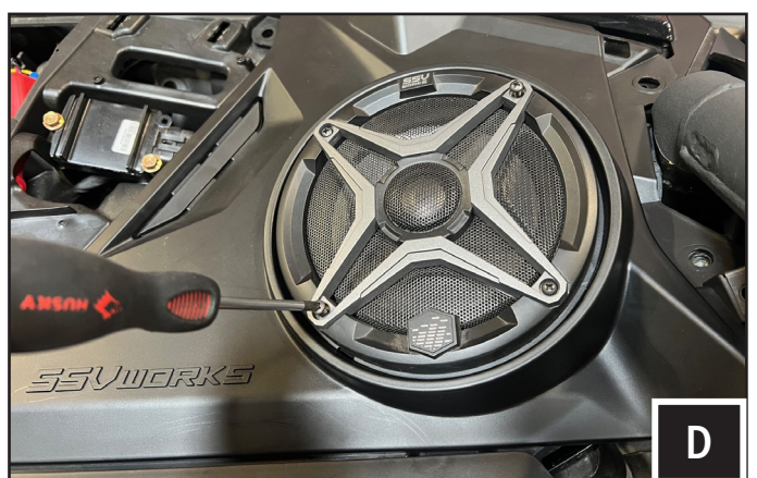
D. Plug in the speaker and mount it to the driver and passenger side Mav R speaker panels using the screws included with the speakers.
