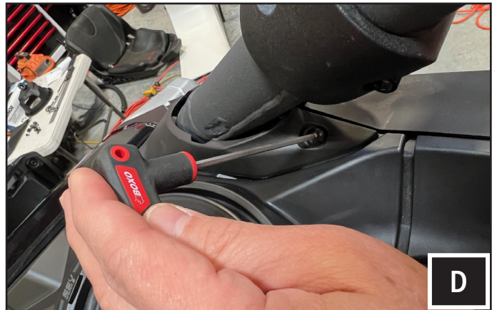
D. Remove the left and right side corner trims using a 3mm allen wrench.
