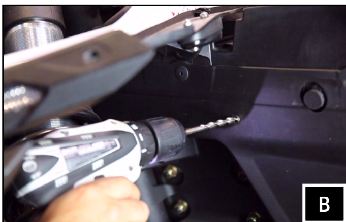
B. Drill a hole through the pilot holes using a 1/4" drill bit. Be sure to move the amp plate out of the way before drilling.
