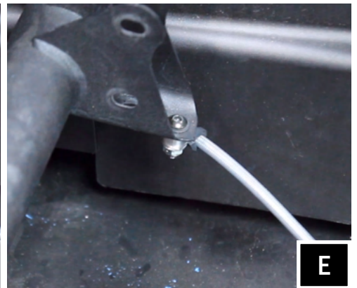
E. Remove the factory 10mm nut and bolt from the brake line. Place the washer on top of the factory bracket and push the long M6x25mm screw through the top. Then attach the brake line, spacer, washer and nut. (Disregard this step for the 4-seat Maverick X3 Max)
