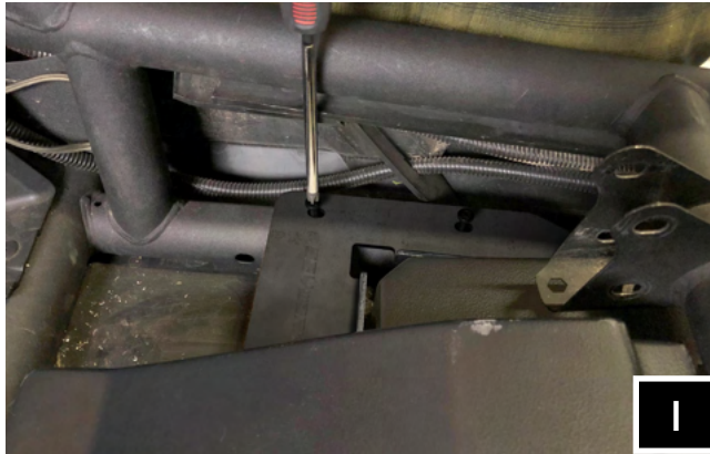
I. The large bracket will align over (2) factory holes in the chassis. Using a #3 Phillips screwdriver, secure the large bracket to the chassis with the provided (2) thread rolling screws and washers.
