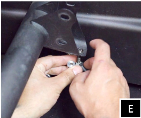
E. Remove the factory 10mm nut and bolt from the brake line. Place the washer on top of the factory bracket and push the long M6x25mm screw through the top. Then attach the brake line, spacer, washer and nut. (Disregard this step for the 4-seat Maverick X3 Max)
