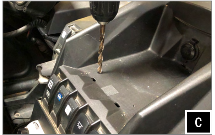
C. Set aside the base plate and open the pilot holes up with a 1/4" drill bit.
