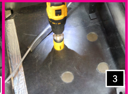
H. To help minimize skid plate rattle, we have supplied a drill template that adds 4 holes to help relieve air pressure that is being generated by the high output of the sub enclosure. Use the mounting bracket for the front of the sub enclosure for reference. Line up the template under the sub mounting brackets. (1). With hole punch/scribe tool mark the 4 drilling points through the template on to the floorboard (2). Drill the four (4) - 1½" holes with a hole saw (3).
