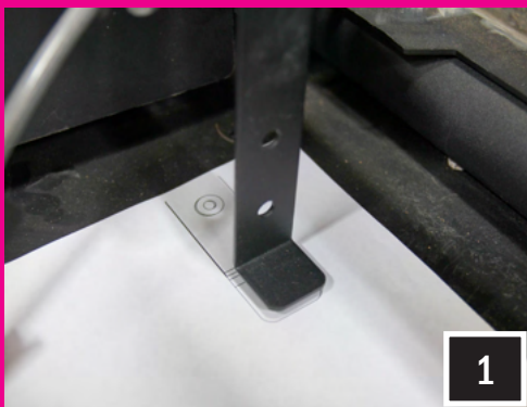
H. To help minimize skid plate rattle, we have supplied a drill template that adds 4 holes to help relieve air pressure that is being generated by the high output of the sub enclosure. Use the mounting bracket for the front of the sub enclosure for reference. Line up the template under the sub mounting brackets. (1). With hole punch/scribe tool mark the 4 drilling points through the template on to the floorboard (2). Drill the four (4) - 1½" holes with a hole saw (3).
