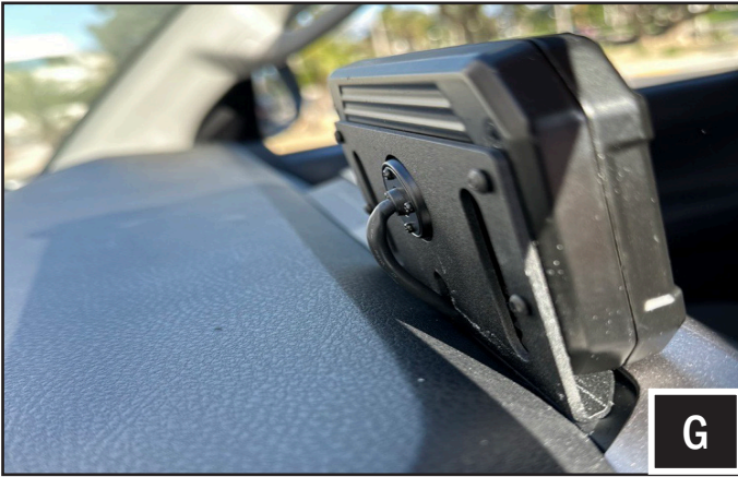
G. Run the controller cable through the notch filed earlier and run the cable towards the driver left corner footwell.
