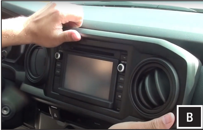
B. Placing one hand on top and the other at the bottom right corner, slowly pull on the bezel while moving your hands around the bezel.
