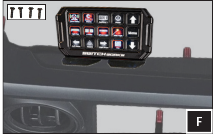
F. Mount the Controller to the B-MB3423 using the thread cutting screws (B-S3262) before re-installing the bezel to the dashboard.
