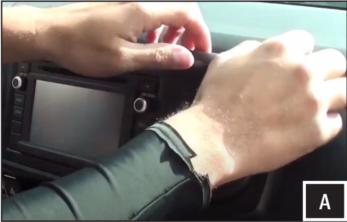
A. Remove the radio trim bezel by carefully pulling from the upper left corner of the bezel.
