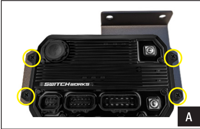
A. Mount the SWITCH Works brain module to the B-MB3203 bracket using the supplied M5x10mm screw (x4).
