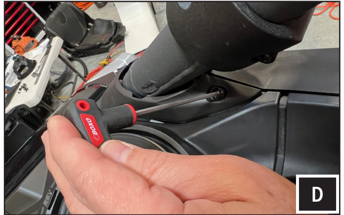
D. Remove the left and right A pillar trims using a 3mm Allen wrench.
