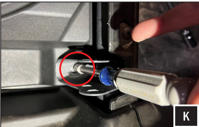
K. Align the front screw holes and use (2) M6x16mm hex head bolts and washer to secure the enclosure.
