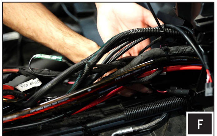
F. Run the rear speaker, subwoofer and RGB cables along the passenger side of the center console. Use zip ties to tidy up the install.
