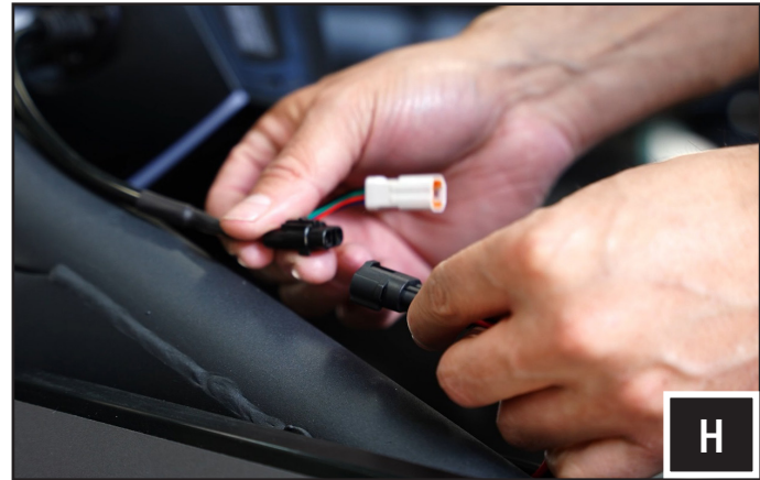
I. Plug in the speaker pod audio and RGB connectors to the B-H2936 rear speaker Y harnesses.
