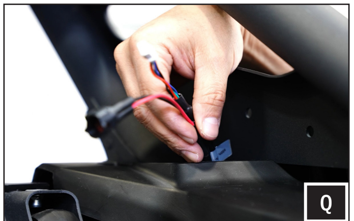
Q. Run the driver and passenger side speaker harness through the plastic panel by the B-pillar.
