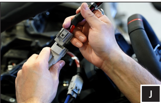
J. Plug in the power connector of the amps to the power cable.
