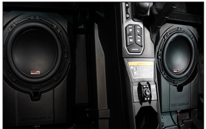
Completed dual subwoofer installation with LIT-CC RGB controller on the center console.
