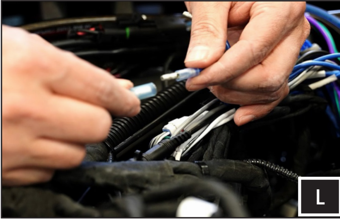
L. Plug in the amplifiers turn-on bullet connectors to the turn-on delay module output wire. See page 7 for reference.
