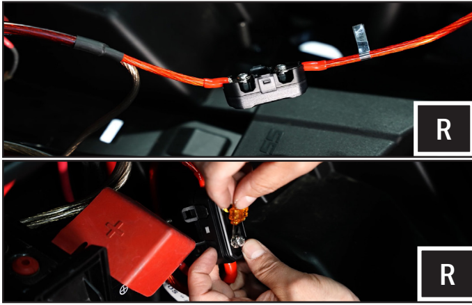
R. Install the fuse holder on the power wire no more than 18" away from the battery and install the fuse.
