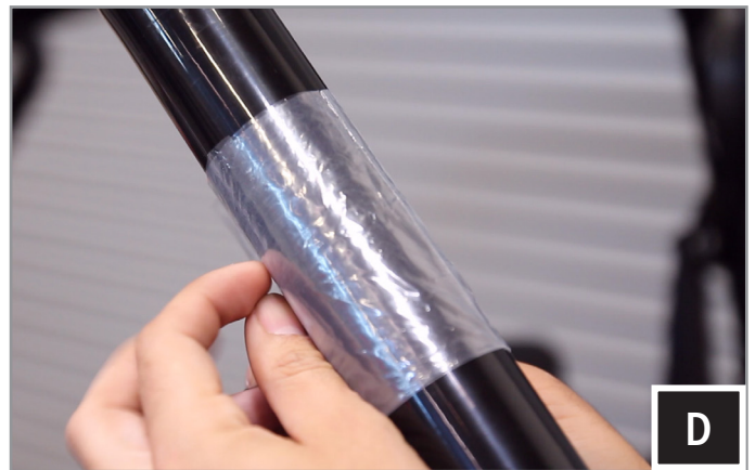
D. Place both ring mounting clamps on the cage using the plastic bag to prevent scratching, place the cage mount pod in its final mounting location and
