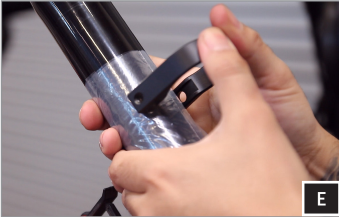
E. Slide the (2) clamps onto the tube.
