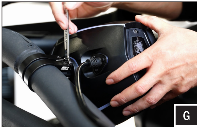
G. Adjust the cage pod to point towards the headrest and tighten the clamp base bolts.
