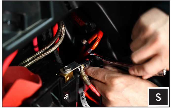
S. Connect the power wire to the battery positive and negative posts.
