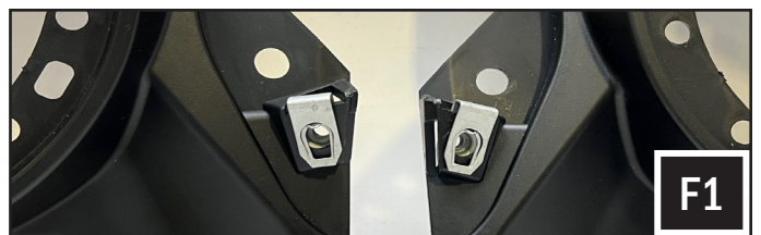
F. Remove u-nuts from the factory panels and install on the Mav R dash panels (F1).
