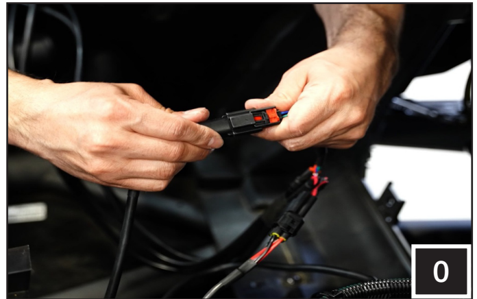
O. Plug in the B-H2936 (rear speaker harness) to the B-H1913 (4-pin audio extension harness, 8 ft.).
