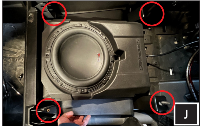
J. Slide the Mav R subwoofer enclosure under the front seat rail mounts and insert the brackets to the rear seat rail studs.
