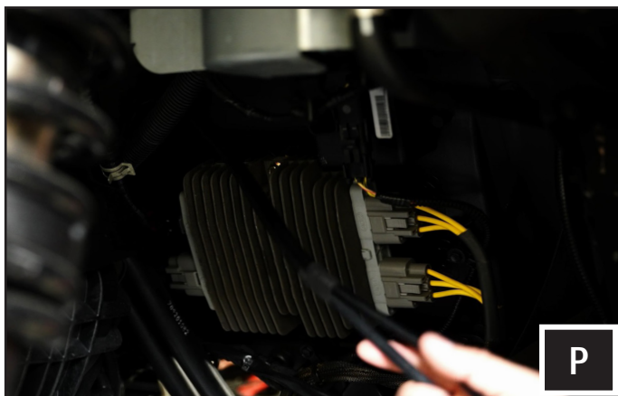
P. Split the B-H2936 rear speaker harness to the passenger and driver side along the rear firewall. Zip tie the cables to the factory harness and avoid hot or moving parts.
