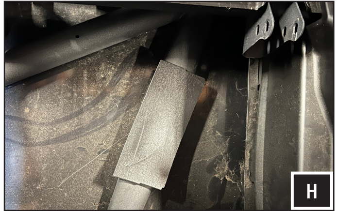
H. Apply the foam pad (included in the kit) to the flat portion of the bottom reinforcement tube.
