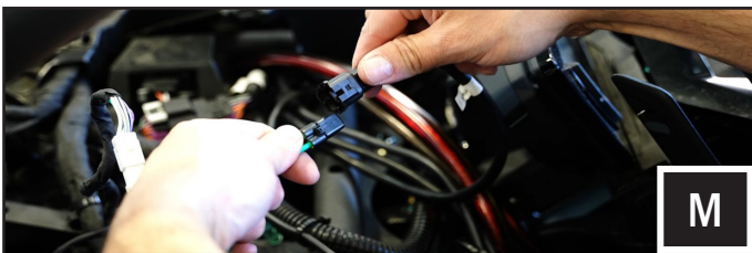
K. Plug in the 8-pin speaker and 2-pin subwoofer input connectors of the amplifiers to the factory radio output wiring.
