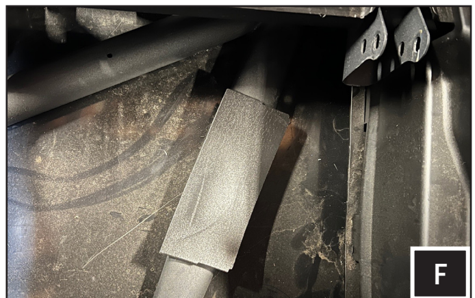
F. Apply the foam pad (included in the kit) to the flat portion of the bottom reinforcement tube.
