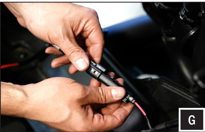
G. Plug in the subwoofer connector to the B-H2702 subwoofer extension cable.
