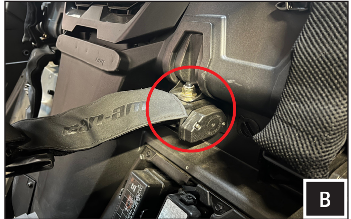
B. If installing the subwoofer enclosure under the driver seat, use an 18mm socket wrench to remove the right shoulder seat belt retractor mechanism. Otherwise, skip to step D.
