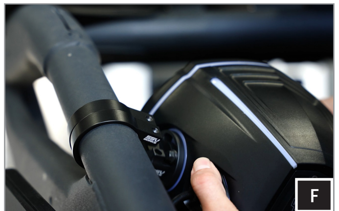
F. Secure to the clamps using the two (2) M6 Allen socket head bolts and washers with a 5mm Allen key.
