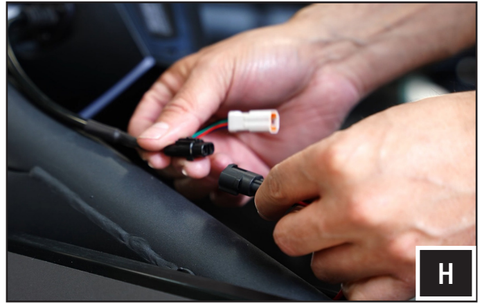
I. Plug in the speaker pod audio connectors to the B-H2936 rear speaker Y harnesses.
