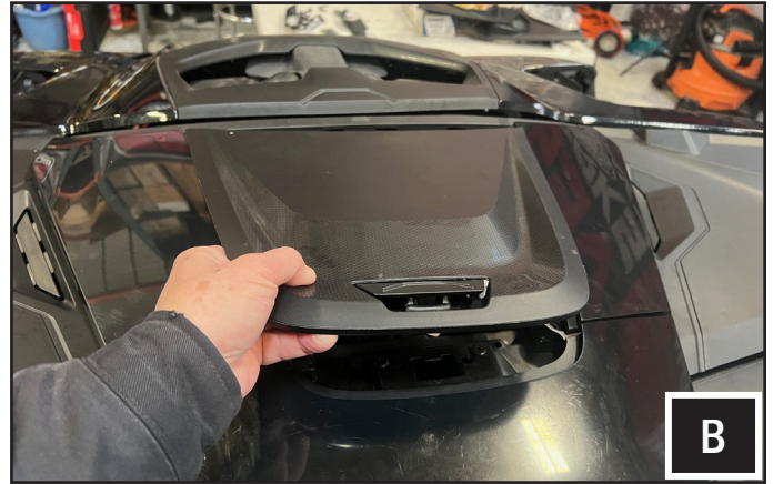
B. Remove the front fuse box cover.
