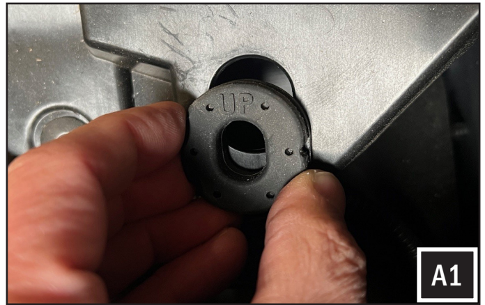
A1. The speaker bucket grommet is designed to be inserted with the "UP" side on top for ease of the installation.
