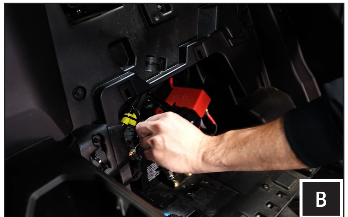
B. Disconnect negative battery terminal.
