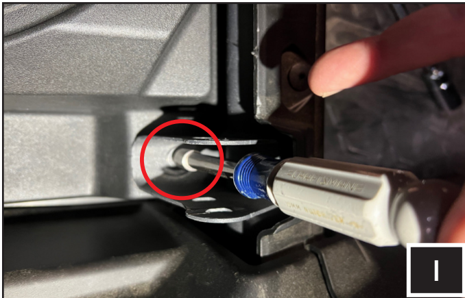
I. Align the front screw holes and use (2) M6x16mm hex head bolts and washer to secure the enclosure.
