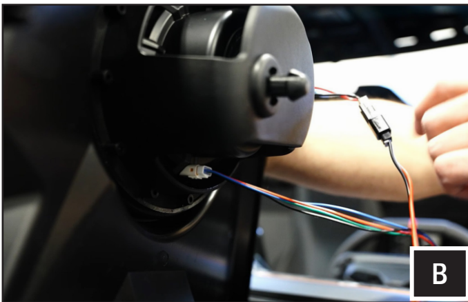
B. Plug in audio connectors of B-H1385 to the driver and passenger side dash panel speakers.
