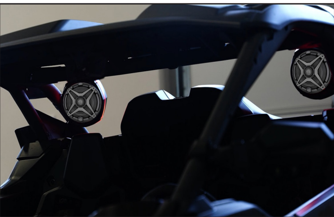
Completed rear speaker pods installation.
