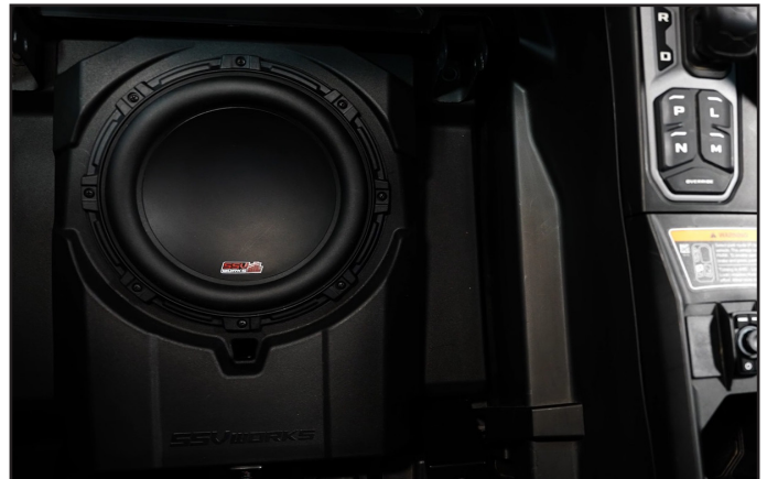
Completed subwoofer installation under the driver seat.
