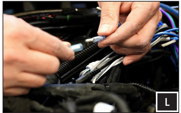
L. Plug in the amplifier turn-on bullet connectors to the turn-on delay module output wire. See page 4 for reference.
