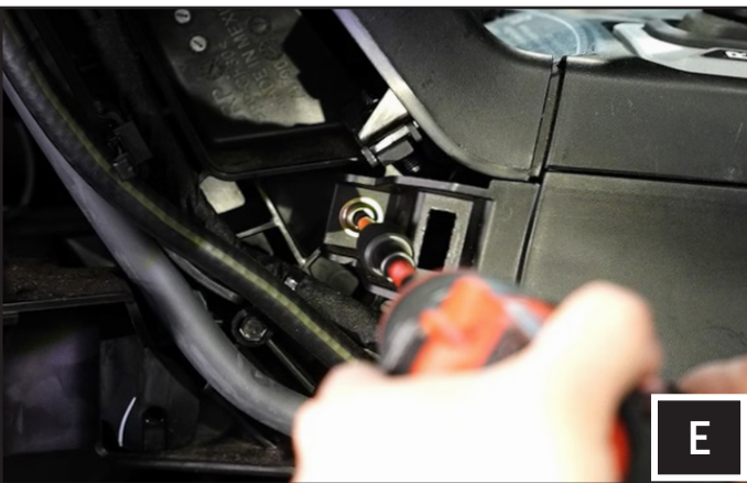
E. Remove the screw to remove the rest of the center console side panel. Do the same for the passenger side panels.
