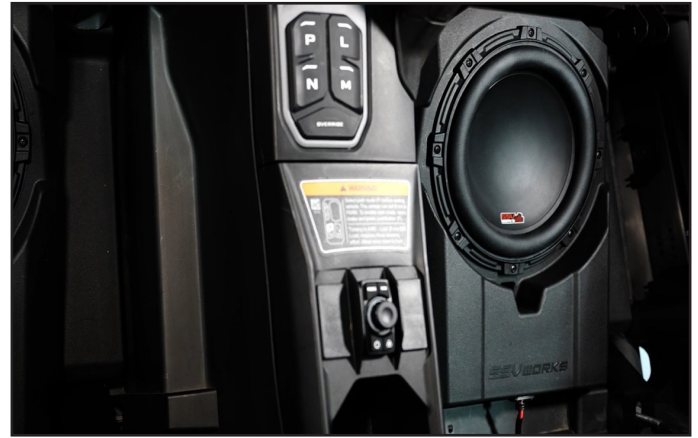
Completed subwoofer installation under the passenger seat with LIT-CC RGB controller on the center console.
