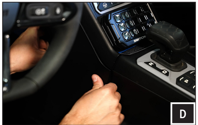
D. Reinstall the center console and other panels removed during installation.
