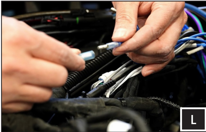
L. Plug in the amplifier's turn-on bullet connectors to the turn-on delay module output wire. See page 6 for reference.
