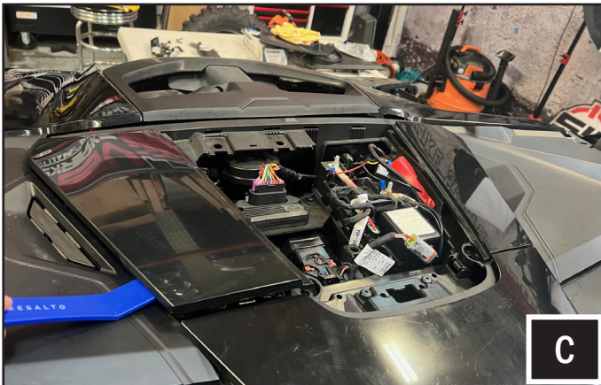
C. Use a plastic pry tool to remove the left and right side center panel trims.
