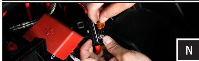
N. Install the fuse holder on the power wire no more than 18" away from the battery and install the fuse.
