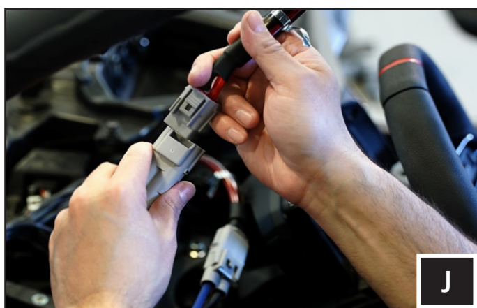
J. Plug in the power connector of the amps to the power cable.
