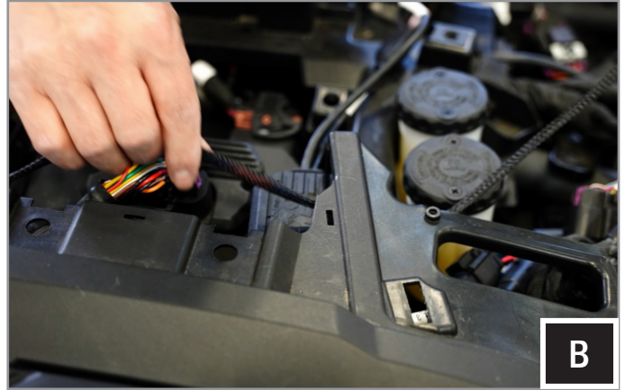
B. Route the turn-on delay output wire towards the steering column.
