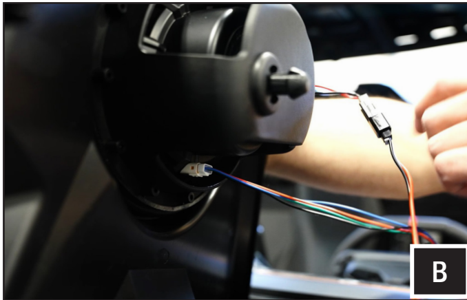
B. Plug in audio and RGB connectors of B-H1385 to the driver and passenger side dash panel speakers.
