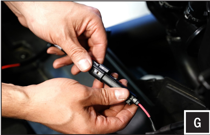
G. Plug in the subwoofer connector to the B-H2702 extension cable.
