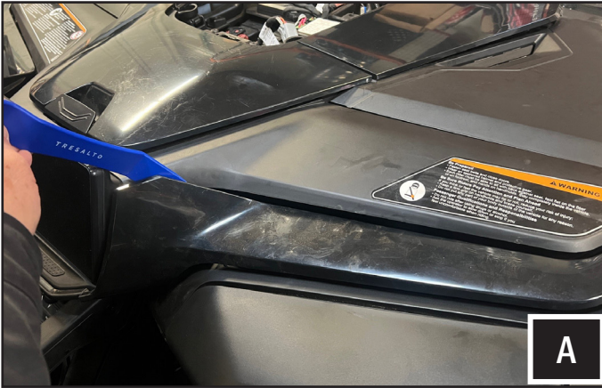
A. Use a plastic pry tool to remove the driver and passenger side front trims.
