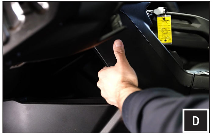
D. Remove the center console side panels.
