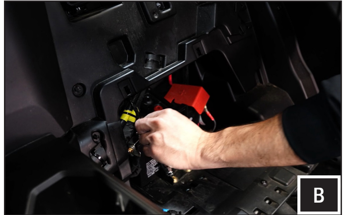
B. Disconnect negative battery terminal.
