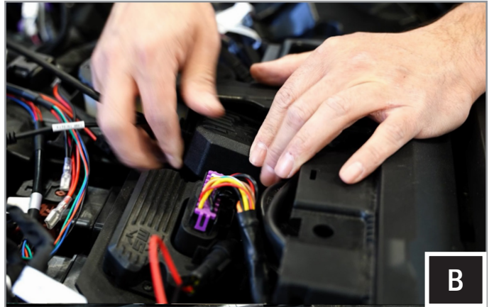
B. Mount the LIT-CC RGB LED Controller Command Center in the dash away from moving parts and secure with zip ties. Cut excess zip ties for a clean install.
