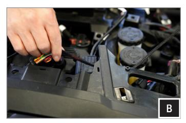
B. Route the turn-on delay output wire towards the steering column.
