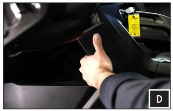
D. Remove the center console side panels.
