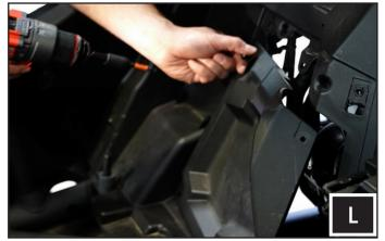
N. Remove the panel behind the passenger seat.
