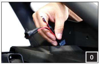
0. Run the driver and passenger side speaker harness through the plastic panel by the B-pillar.
