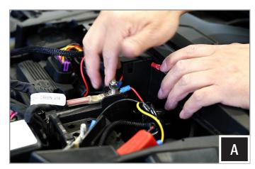
A. Connect the amplifier turn-on delay module's power and ground wires to the factory bus bar. Secure the module to a harness using zip ties.
