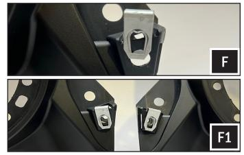
F. Remove u-nuts from the factory panels and install on the Mav R dash panels (F1).
