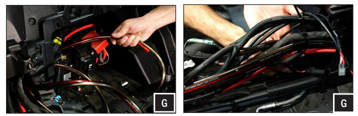
G. Route the power cables along the driver side center console from the battery location towards the driver side dash.
