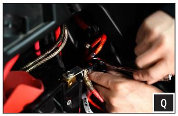
Q. Connect the power wire to the battery positive and negative posts.
